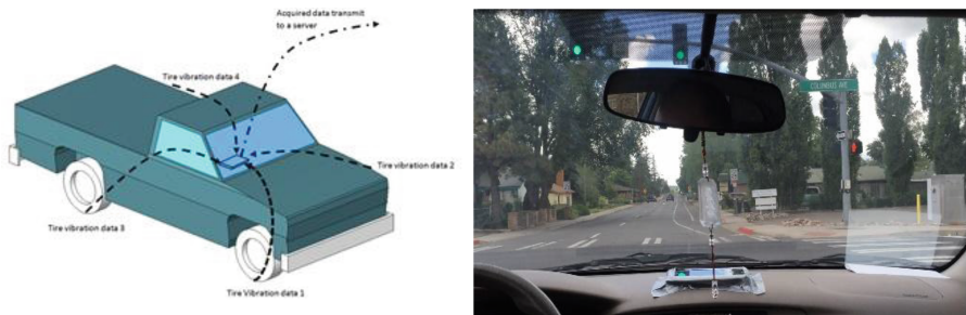
Fig. 2. Schematic of vibration data and placement of a smartphone
