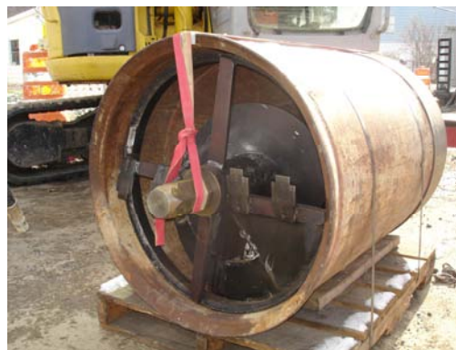
Figure 11- 2 step Reaming Head- Front view (29 inch OD)
