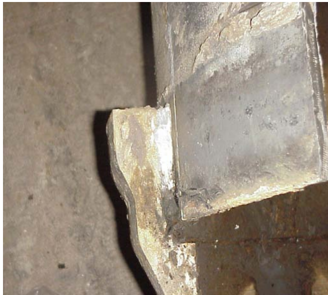
Coupon removed from the cast iron water line. Cut-through of bell/spigot joint showing leak caulking
