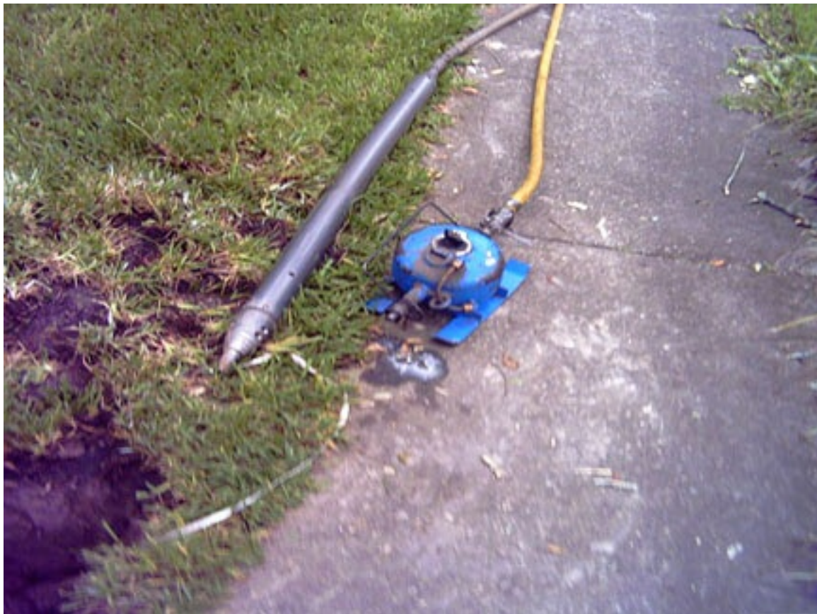
Figure 4 A typical piercing tool setup includes the boring tool, reinforced air hose and lubricator. Compressed air supply is provided by a typical construction air compressor.
