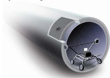
Figure 2. Electromagnetic Inspection of Large Diameter Mains
