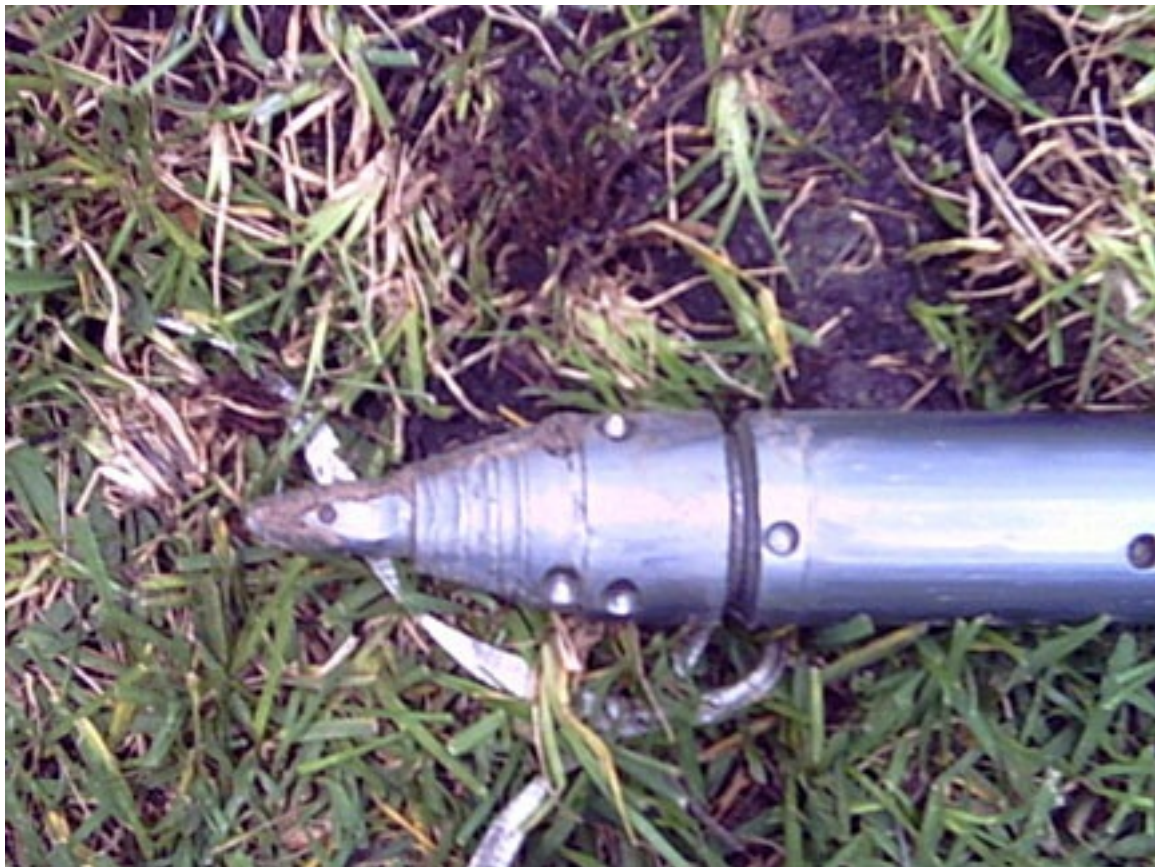
Figure 3 This illustration shows a well-used piercing tool, note the wear on the chisel and stepped cone. These can be replaced at the discretion of the user.
