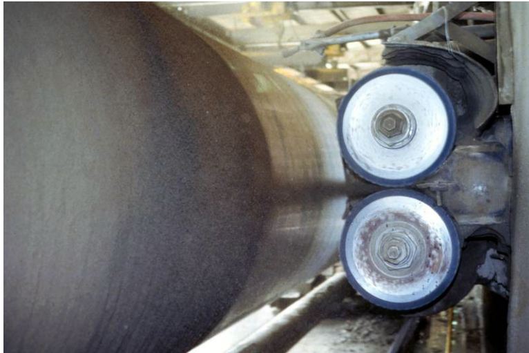
Figure 3. Cement-mortar Coating impaction with two counter rotating rubber brushes.
