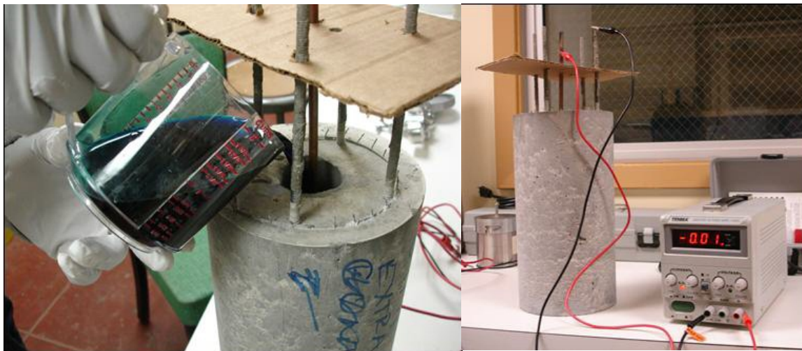
Figure 3. cuprous oxide lactate solution poured into the a specimen (left); The electrokinetic coating process underway, note the copper electrode at the center of void (right)
