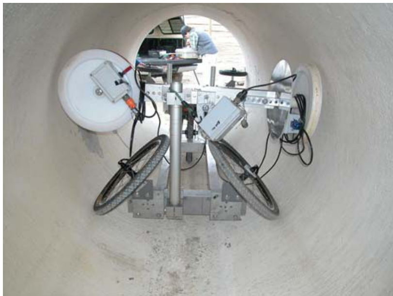
Figure 4 –Magnetic testing introduced in 1997. Manned equipment requires safe pipeline access (Pure Technologies photo)
