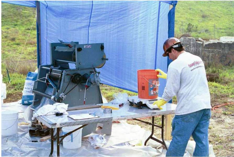
Figure 2 - weighing the saturated material
