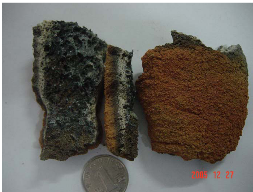
Figure 3 The glass-like casing/liner of the borehole
