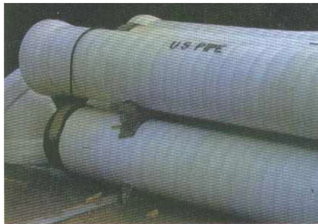
Figure 5. Tape-coated Ductile Iron Pipe (Szeliga/Lieu, 2002)
