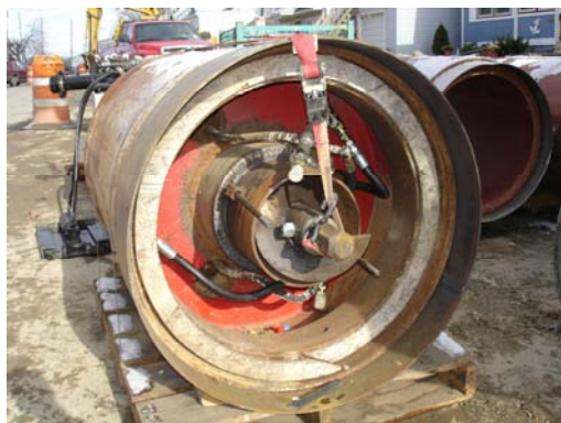
Figure 10- 2 step Reaming Head- Rear View (29 inch OD)
