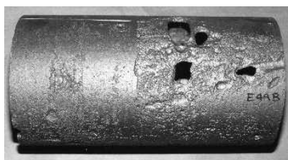
Figure 2 27-year old DI pipe with no protection (after cleaning).
