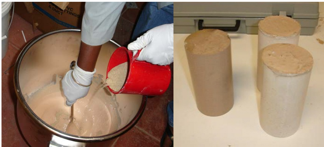
Fig. 1. Metakaolin-based geopolymer paste (left-hand side); Geopolymer cylinders 30 min following casting; notice smoothness of outer surface (right-hand side)
