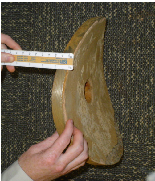
Coupon removed from the cast iron water line. Cut-through of bell/spigot joint showing leak caulking
