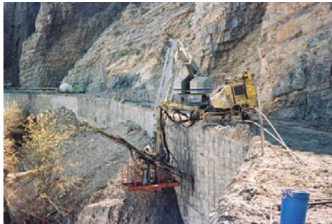
FIGURE 13 Pull-testing rock bolt on steel plate at face of textured wall.
