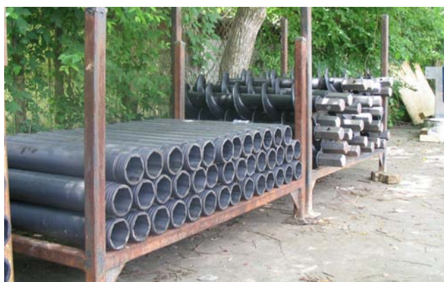
Figure 5- Hollow steel pilot tubes (4 inch diameter)
