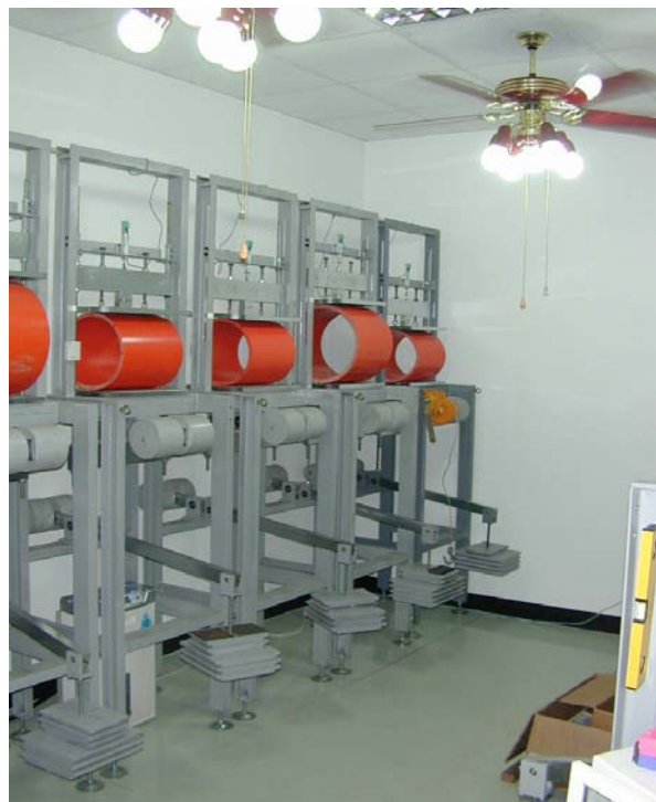
Figure 1 Setup of the long-term pipe stiffness test apparatuses.
