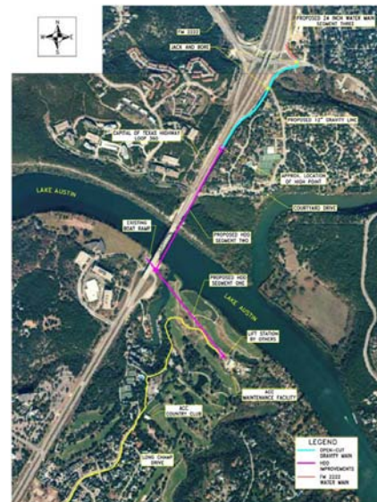
Figure 1 – Davenport Ranch HDD Site: The two combined Horizontal Directional Drilling (HDD) segments (shown in pink) exceed 4,000 feet of subsurface improvements, installed with no disruption to the golf course, Lake Austin, the public boat ramp, or to Loop 360 and the Pennybaker Bridge.
