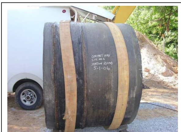
FIGURE 3 4.5-ft Sample (with complete lap joint) cut from 72-inch Pipeline for Lab Analysis
