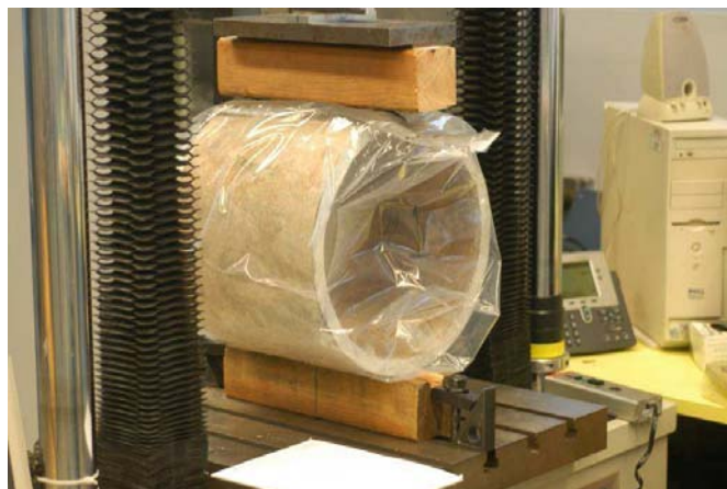
Photo 3 - Three-edge bearing strength test of 14 in. diameter AC pipe.
