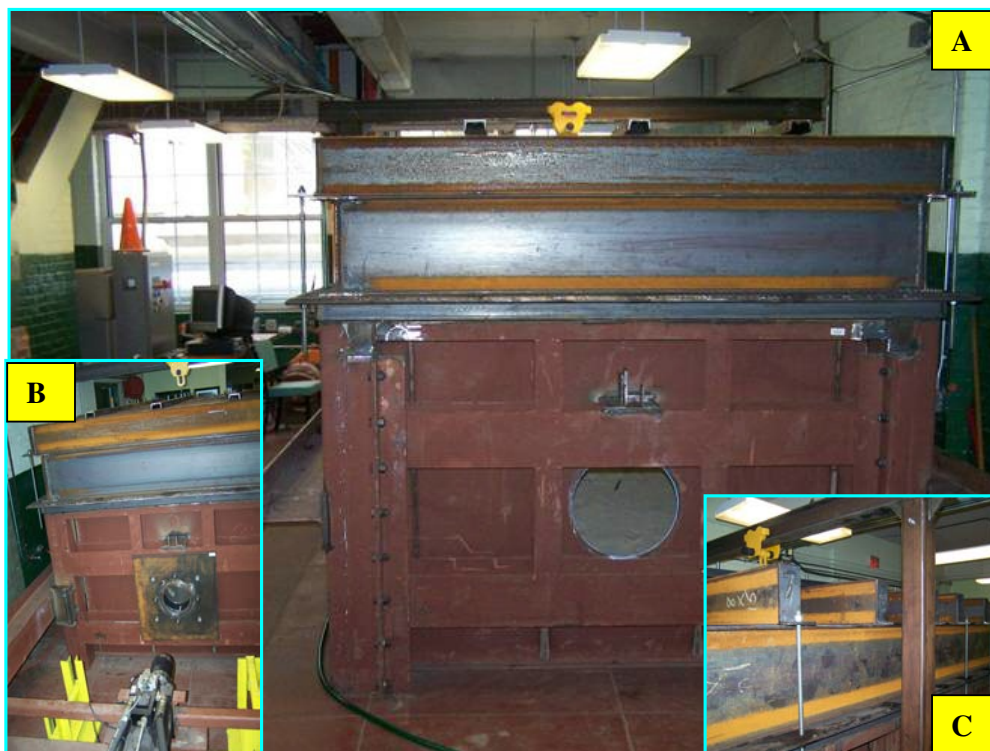
Fig. 7. TTC Soil Structure interaction testing facility; a) View from the rear including control station; b) Front view including servo-control actuator; c) Overhead crane, top beams and tie-down rods
