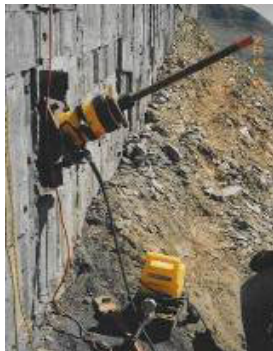
FIGURE 13 Pull-testing rock bolt on steel plate at face of textured wall.
