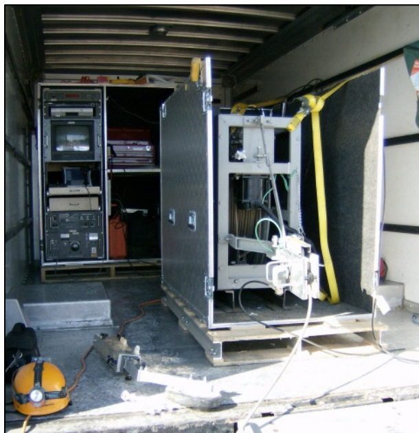
Figure 2. Communication system (left) and umbilical spool (right) stored in van
