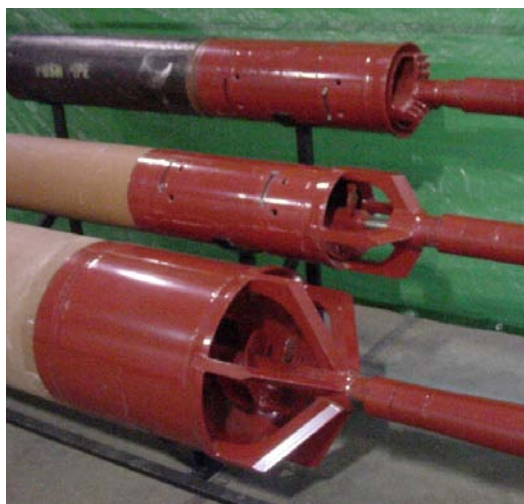
Figure 12- Types of reaming heads. Top- Rotating cutter head Middle and Bottom- conventional knife style
