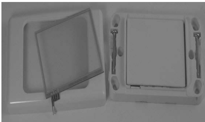
Figure 8-7. Wall plate with removed piece glued back in place behind its original location
