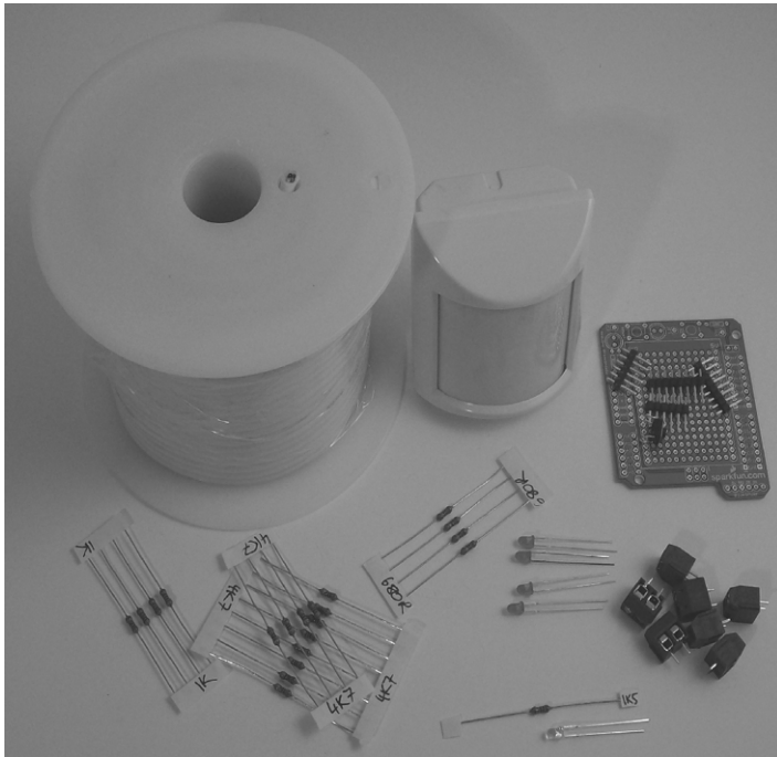
Figure 6-1. Parts required for security sensor inputs
