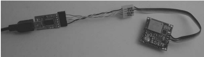
Figure 15-15. The LS20031 GPS module connected to a host computer using an FTDI adapter
