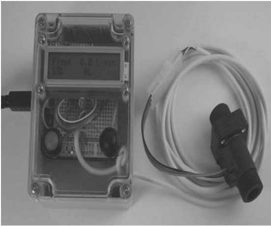
Figure 10-8. Assembled unit with sensor connected
