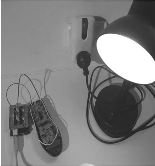
Figure 2-14. Arduino and shield using an appliance remote control to activate a lamp
