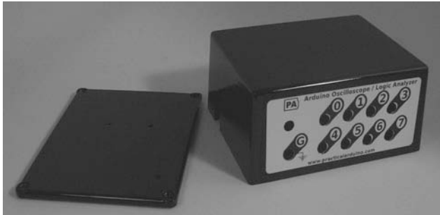
Figure 11-5. Front panel label in place with holes drilled
