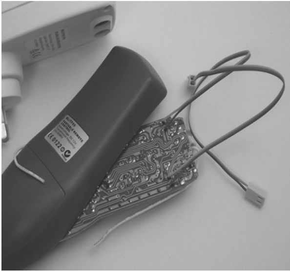
Figure 2-11. Remote control transmitter with connections in place
