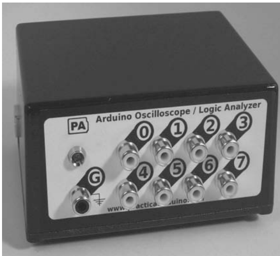
Figure 11-6. Connectors and LED mounted in front panel
