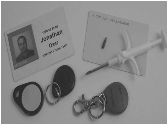
Figure 14-2. RFID tags in a variety of form factors including access cards, key fobs, and a surgically implantable pellet
