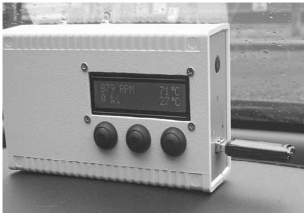
Figure 15-32. The complete system assembled in a case with USB memory stick attached
