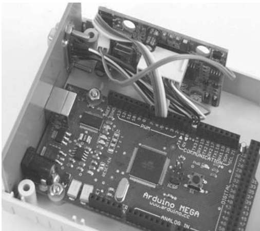
Figure 15-26. The Arduino Mega mounted on plastic spacers with the USB socket protruding through the back panel
