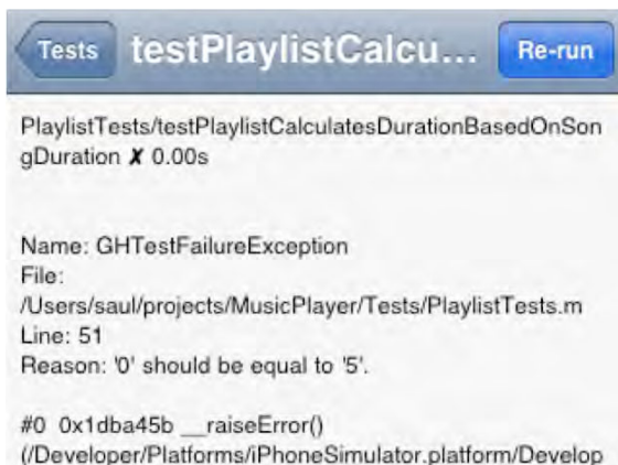
Figure 4–18. The test failed since the return value of the duration method is 0. Your test expects the return value to be 5.
