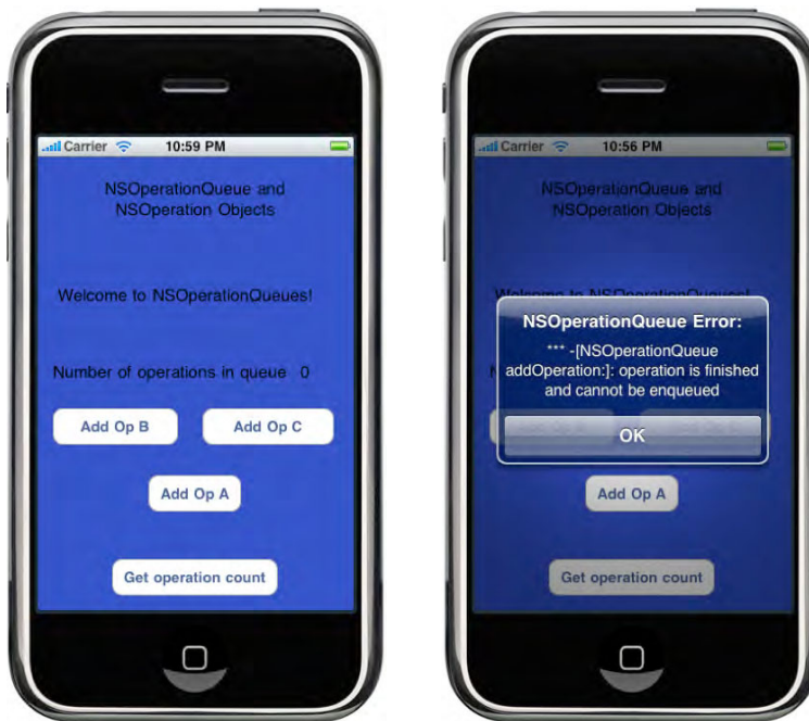
Figure 1–14. Adding operation objects to an operation queue and the result of adding an operation to a queue after it has finished executing.
