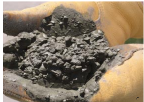
Figure 5. Samples of pervious concrete with different water contents, formed into a ball: (a) too little water, (b) proper amount of water, and (c) too much water. [IMG15595, IMG15596, IMG15597]
