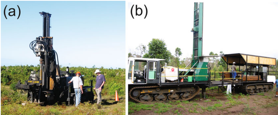
Fig. 4.33 Sonic drill rigs: (a) track mounted light rig for drilling shallow holes, up to 30 m deep; (b) heavy duty rig allowing to drill holes more than 100 m deep
