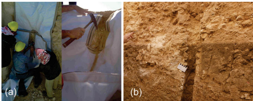
Fig. 5.2 Channel sampling of the exploration trench walls. Uranium deposit in central Jordan: (a) channel sampling using hammer and chisel; (b) channel sample cut by diamond saw
