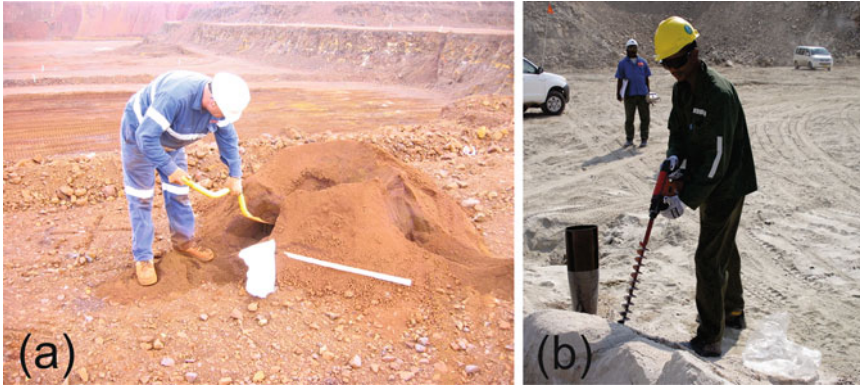
Fig. 4.24 Blasthole cone sampling for grade control purpose: (a) sampling by shovel, Yandi iron-ore mine, Western Australia; (b) sampling by hand held auger drill, Rossing uranium mine, Namibia
