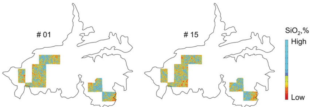
Fig. 28.2 Two equiprobable realisations (#01 and #15) of the SGS model showing spatial distribution of the SiO 2 (%) grade. The model was built using the data distributed
