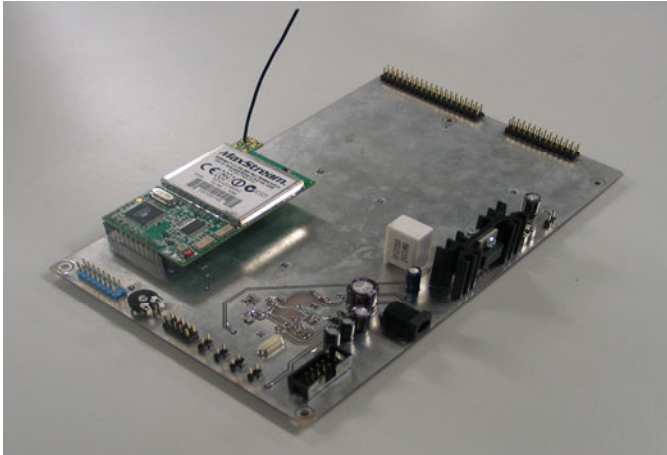
Fig. 8.22 Completed firing system board with attached RF module
