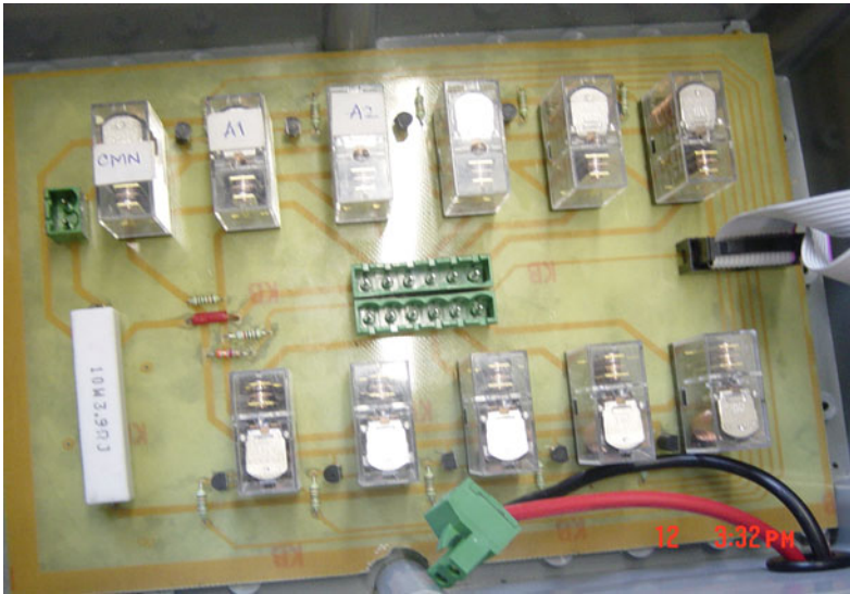
Fig. 8.2 Initial design of a 10-channel detonator board
