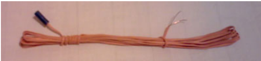
Fig. 8.8 An electric match used for detonating fireworks
