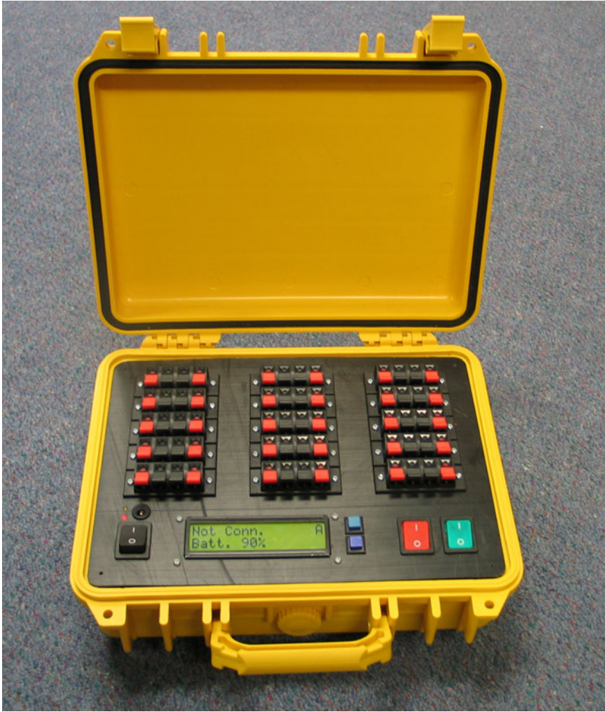
Fig. 8.24 Enclosure and hardware control panel
