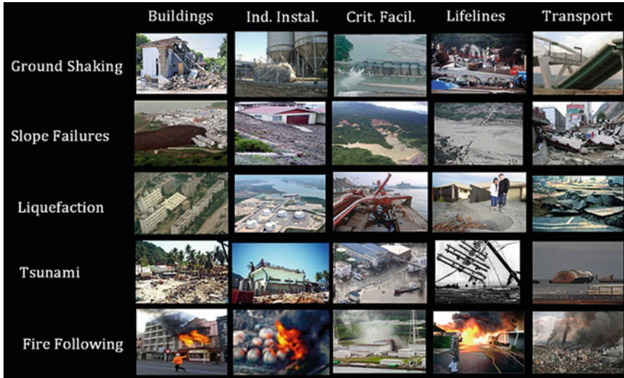
Fig. 1.18 Types of earthquake consequences considered in the GEM Earthquake Consequences database (So et al. 2012)
