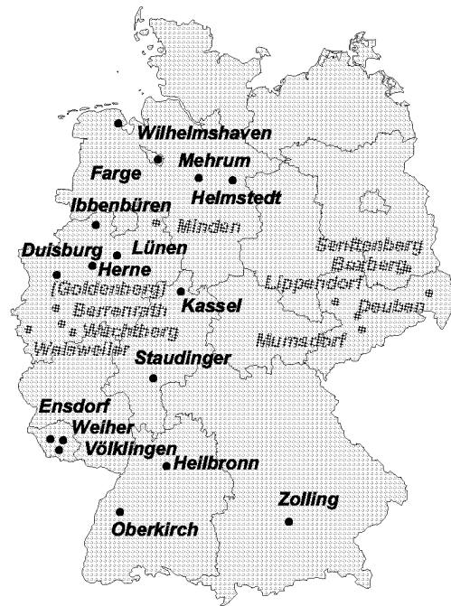
Fig. 10 Locations of power stations with co-firing of sewage sludge (bituminous coal firing in black, lignite firing in grey; from [32])
