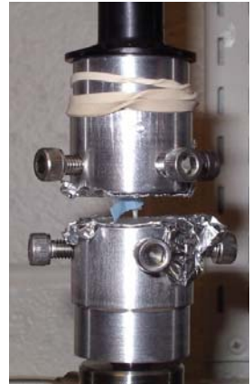
Fig. 4. A murine mouse tibia loaded within the testing apparatus
