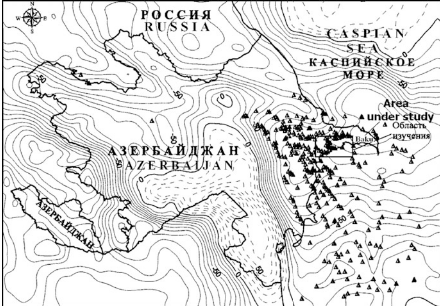
Fig. 8.1 Distribution of mud volcanoes ( black triangles ) in the Eastern Caucasus and Bouguer gravity data (Kadirov and Mukhtarov 2004). Isoanomals (in milliGals): solid lines denote negative values, dashed lines denote positive values
