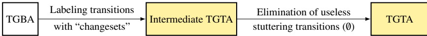
Fig. 3. The two steps of the construction of a TGTA from a TGBA
