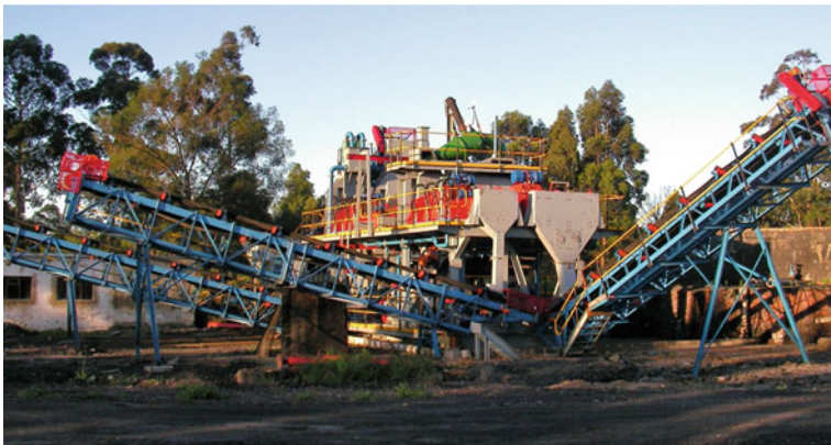
Fig. 3.15 Mobile wash plant with 100 tons/h feed capacity in South Africa (Source: Author's photograph)
