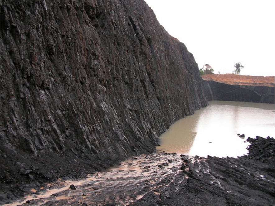
Thirty-meter low-rank coal seam in Kalimantan, Indonesia
