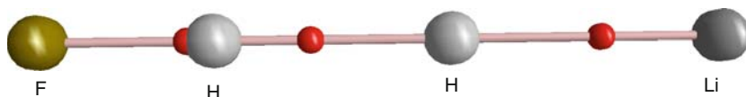
Fig. 12.5 Molecular graph of the F–H⋯H–Li complex, big circles correspond to attractors, small red circles to BCPs, the BPs are also given ( pink lines )
