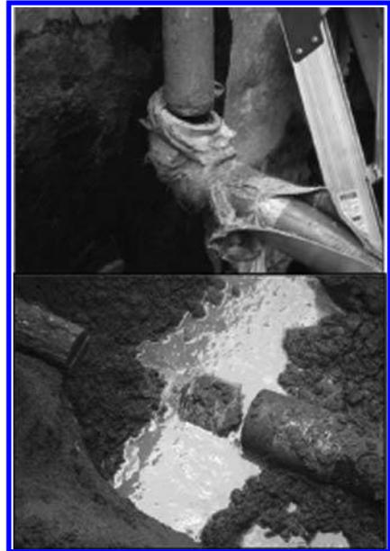
Figure 35. Damage to buried pipes occurred to fire protection pipe lines buried in backfill soil around the buildings (Sakai et al., 2009).
