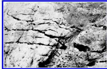
Figure 5. Ground fissure developed in soft soil ground.
