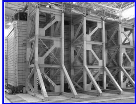
Figure 5. Laminar box before shaking.
