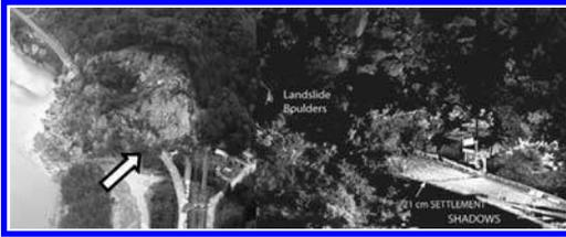
Figure 2. The reconnaissance for the 2004 Niigata Ken Chuetsu earthquake in Japan provided geo-engineers an opportunity to use new technologies in their field studies. Aerial photography and terrestrial LIDAR were used to document earthquake-induced landslides, such as the Shiroya Slide, which is shown here (Rathje et al., 2006).
