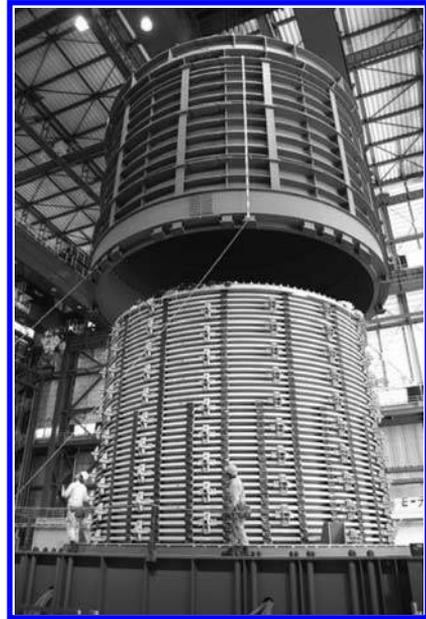
Figure 24. Laminar box being covered for saturation.
