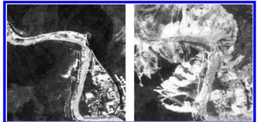
Figure 3. Pre- and post-earthquake VHR satellite imagery of landslides and building damage induced by the 2008 Wenchuan earthquake in the town of Ying Xiu, Sichuan Province, China.
