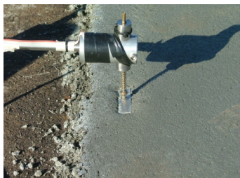
JDMD Placed at the Edge of the Concrete
