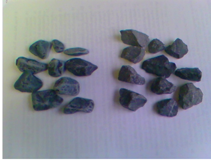
FIG. 1. Aggregate particles after Micro-Deval (left) and before Micro-Deval (right)
