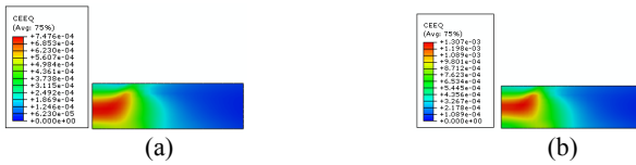
FIG.18. Equivalent creep strain contours in asphalt layer under different traffic loading level: (a) 100 kN, (b) 200 kN
