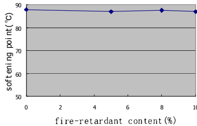
FIG.5. relationship of fire-retardant cont. with soft point
