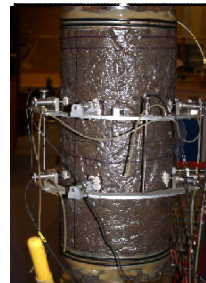
FIG. 5. Haversine triaxial repeated loading curve (left) and instrumented triaxial specimen ready for testing (right)
