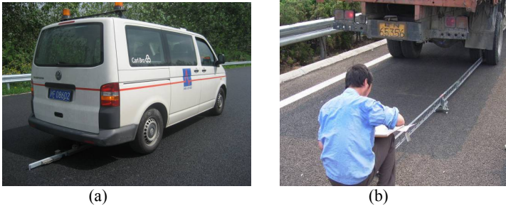
FIG. 3. Devices used in structure capacity evaluation: (a)FWD and (b)BB
