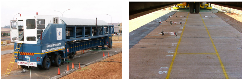
FIG. 4. HVS with its dual wheel loading configuration
