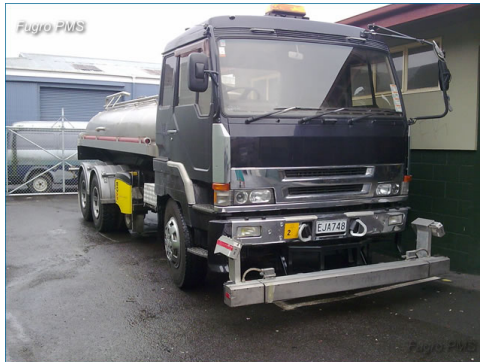
FIG. 1. Norsemeter ROAR MkII survey equipment
