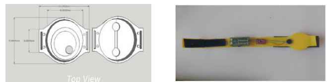
Fig. 1 Alerting bracelet case design (left) and completed prototype (right)
