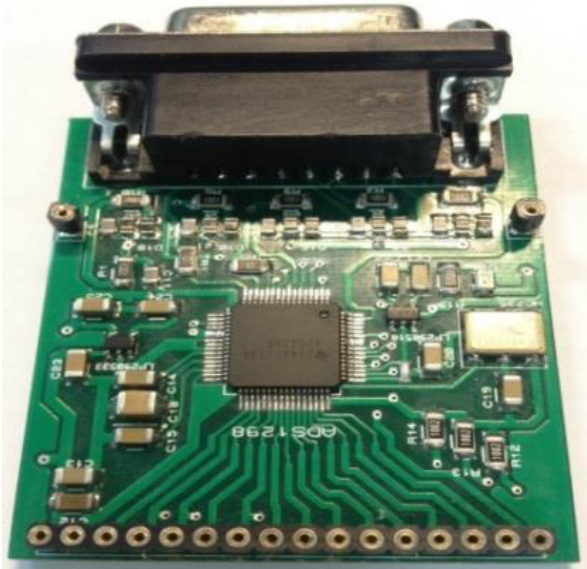
Fig. 8 Practical implementation of the proposed ECH front-end device
