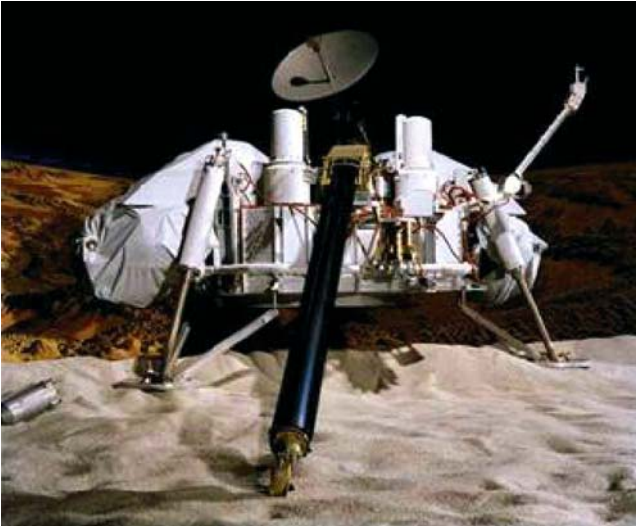
Fig. 13.23. One of the Viking landers with its mechanical arm deployed (photo courtesy of NASA/JPL)
