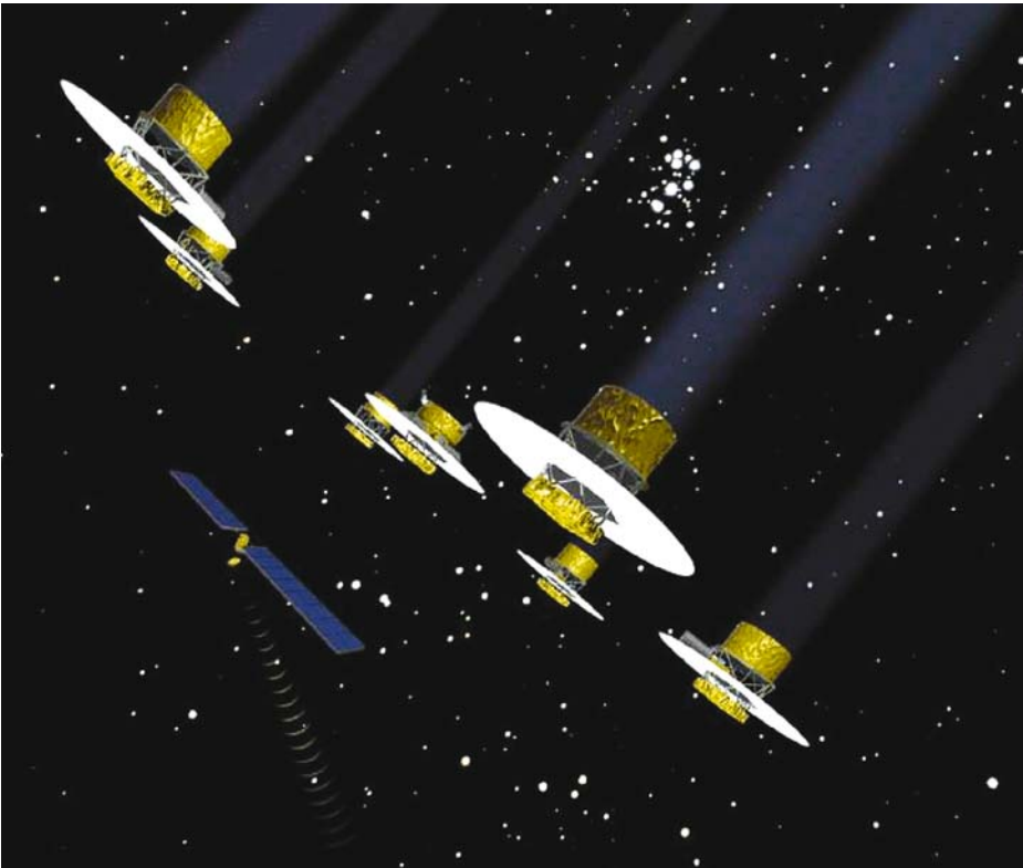
Fig. 6.18. Artist's representation of the DARWIN mission, seen in a six-telescope circular configuration. The central satellite is the beam combiner. An eighth satellite, out of the flotilla plane, allows for information transfer to the Earth and the metrology of the array (from an ESA study realized in 1998 by Alcatel Space Industries)
