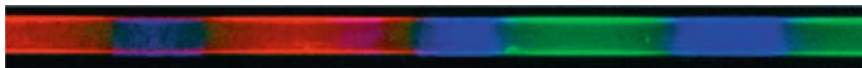
Fig. 29 A barcode of three different chemical functionalities formed in a silica capillary via spatially-selective polymerization. It consists of segments of poly(bis-SorbPC) doped with Rhodamine-capped DPPE ( red ), poly(bis-SorbPC) doped with NBD-capped DOPE ( green ), and DOPC doped with \text{Ni}^{2+} -charged DOGS-NTA. After the lipid pattern was formed, 6xHis-tagged Cerulean, a blue fluorescent protein, was injected into the capillary and bound selectively to the immobilized \text{Ni}^{2+} ( blue ). The capillary inner diameter is 50\ \mu\text{m} . Reprinted with permission from [96]. Copyright 2007, American Chemical Society
