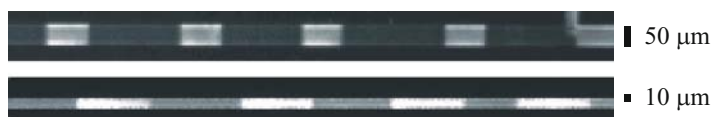
Fig. 13 Fluorescence images of 50 and 10 μm inner diameter capillaries patterned with alternating segments of poly(bis-SorbPC) and 1:50 (mol/mol) Rhodamine-capped DPPE:DOPC. Reprinted with permission from [96]. Copyright 2007, American Chemical Society
