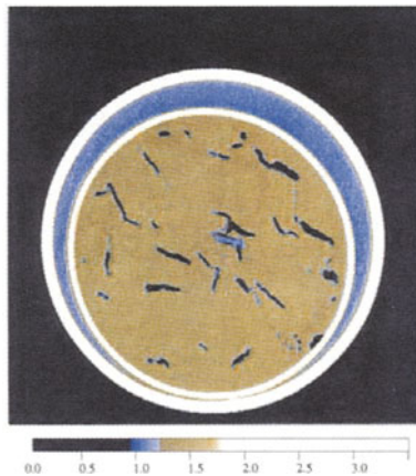
Fig. 3.20. A reconstructed slice from a medical CT scan showing the distribution of methane gas bubbles from a sediment core collected from center of a pockmark in Eckernförde Bay, Baltic Sea (see Figs. 3.15 and 3.18). False colors, based on X-ray densities, represent water (blue), sediment (brown), core liner (white), and methane bubbles (black). The core has been maintained at in situ temperature and pressure (see [Abegg and Anderson 1997] for details).
