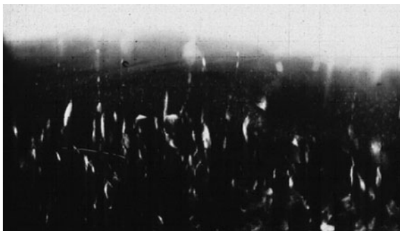
Fig. 3.19. X-radiograph of a 2.5-cm-thick section of sediment (approximately 10 by 20 cm) collected by divers during summer months from the gassy sediments of Cape Lookout, North Carolina [Martens and Klump 1980]. Large methane bubbles appear as white (less dense) objects in this positive X-ray. Note the open bubble tubes (light gray) leading to the sediment–water interface.
