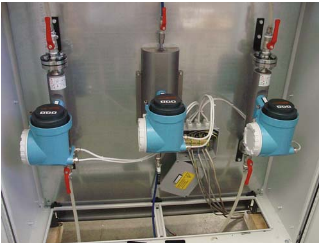
Fig. 18.19 Modern mass flow metering system for a continuous mixer for no-bake sand Source: IMF Luino, Italy and Indianapolis, IN, USA
