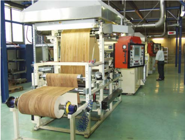
Fig. 11.4 Pilot impregnation line from company VITS at Dynea Austria GmbH, Krems, Austria
