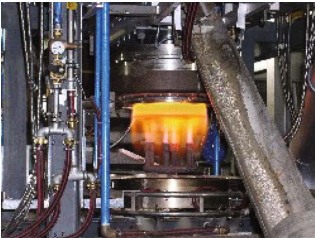
Fig. 10.3 The fiberizing is done in the spinner
