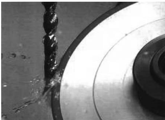
Fig. 13.25 Photo of a diamond grinding wheel in use (photo: Noritake company limited co., Ltd, Japan)
