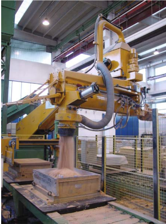
Fig. 18.18 Modern continuous mixer for no-bake sand Source: IMF Luino, Italy and Indianapolis, IN, USA
