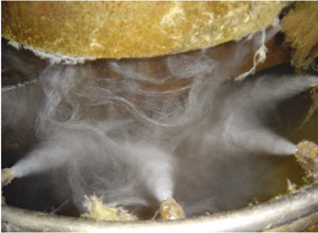
Fig. 10.4 Glass fibers are sprayed with binder
