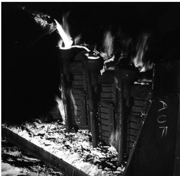
Fig. 18.13 Production of camshafts by the shell molding process
