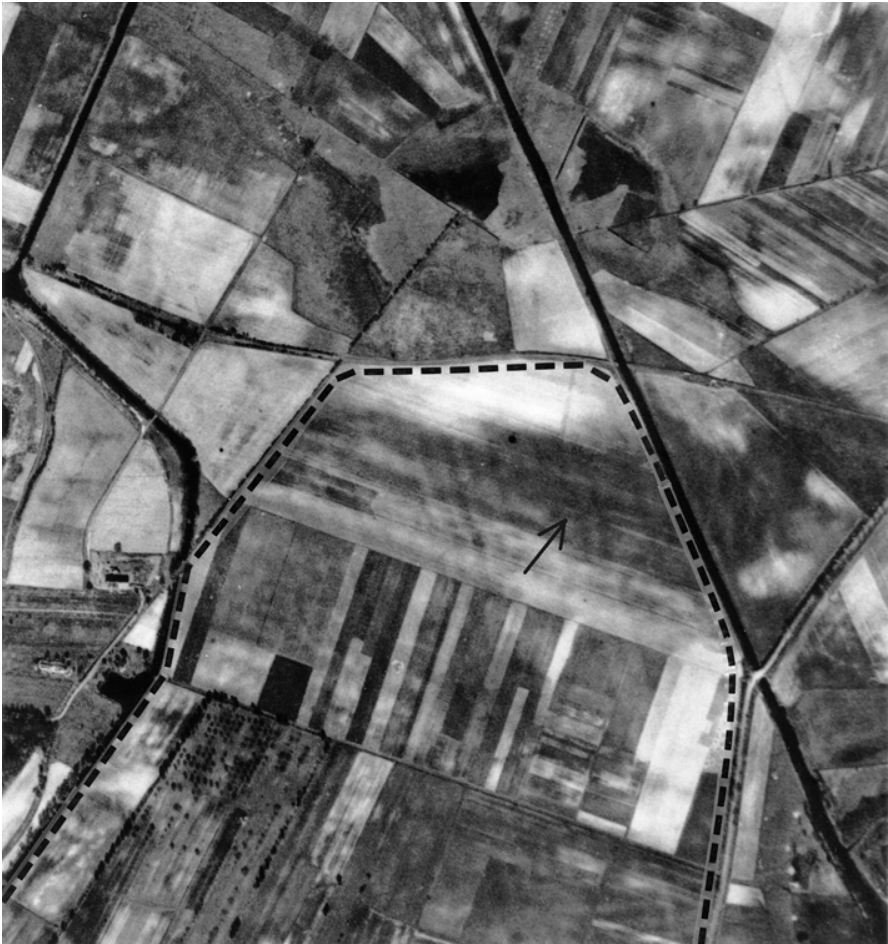
Fig. 3.1-13: Wartime aerial photograph taken on April 10, 1945, showing cultivated land now covered by the northern part of the Schöneiche landfill ( within dashed line ). The high contrast reveals differences in moisture content and lithology. Faint stripes ( arrow ) suggest the presence of an old drainage system or long-term agricultural use (old field patterns). (Courtesy of Luftbilddatenbank, Ing.-Büro Dr. Carls, Estenfeld)
