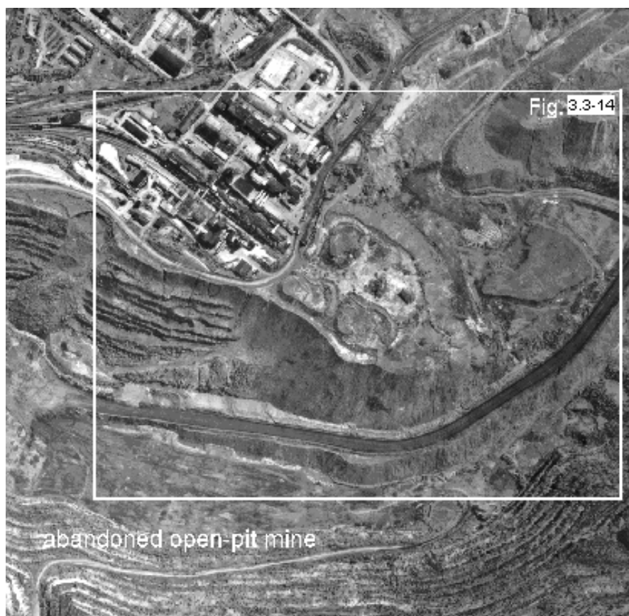
Fig. 3.3-13: Aerial photo taken April 24, 1995, showing a mining landscape in Thuringia, Germany. The dominant landscape structures include part of an abandoned open-pit mine (being filled with tailings), waste heaps, and an abandoned smelting plant (Source: Landesvermessungsamt Thüringen).
