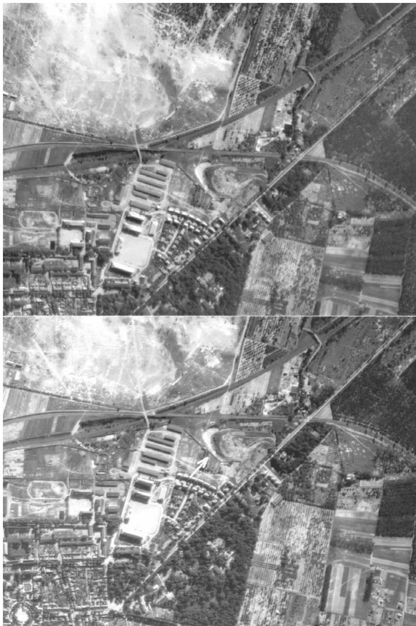
Fig 3.1-10: Archive aerial photograph (stereo-pair) taken on May 28, 1953, showing a deep gravel pit (arrow) at the location of a now abandoned waste disposal site southeast of Ludwigslust ( Fig. 3.1-9 ). Direct dumping of waste into the pit provides direct pathways for contaminated leachate into the uppermost aquifers (source: uve GmbH Berlin)
