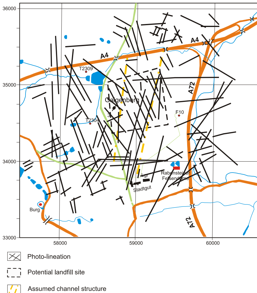
Fig. 6.2-14: Planned waste disposal site at Rabenstein near Chemnitz, Germany: Lineaments derived from b/w aerial photographs from 1988 (TU Bergakademie Freiberg, 1993, commissioned by BGR)
