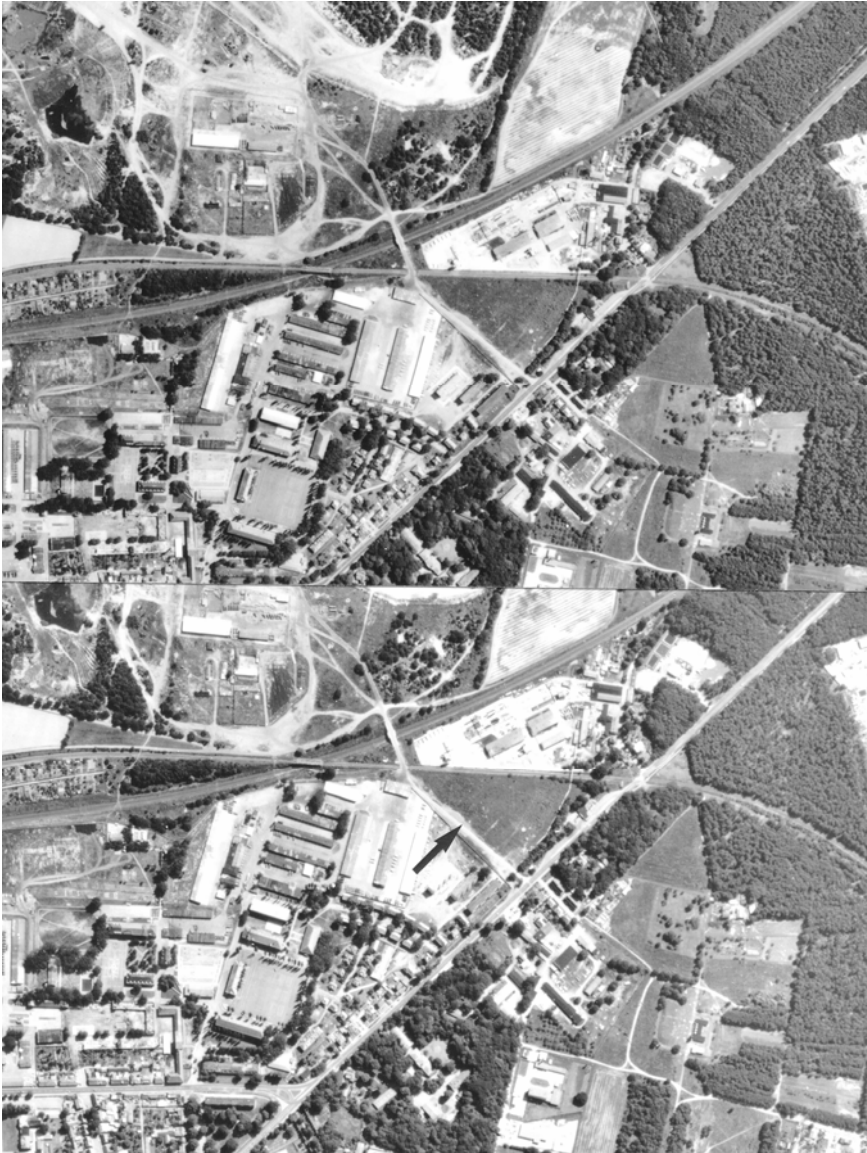
Fig. 3.1-9: Aerial photograph (stereo-pair) taken on July 7, 1991, showing a disused waste disposal site (arrow) southeast of Ludwigslust in Mecklenburg-Vorpommern, Germany. The presently covered and partially overgrown waste site slightly rises above the surrounding terrain (printed with courtesy of the Amt für Geoinformationswesen der Bundeswehr in Euskirchen, Germany). Luftbild © AGeoBw, 1991 - Lizenz B - 7A004
