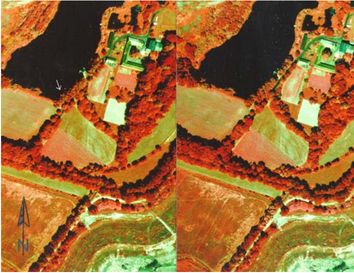
Fig. 3.3-17: CIR aerial photograph taken on July 3, 1993, (stereo-pair) showing an abandoned landfill (area in the center just below the body of water) between the Schöneiche and Schöneicher Plan landfills (Photo taken by WIB GmbH Berlin for BGR)
