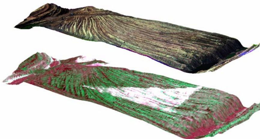
Fig. 3.3-24: An image produced for visualization by the merging of data from different sources. A high-resolution HRSC-A image (top) and a false color HyMap image (bottom) are draped over the HRSC-A DEM. The white areas (bottom) show strong indications of hydrocarbon absorption
