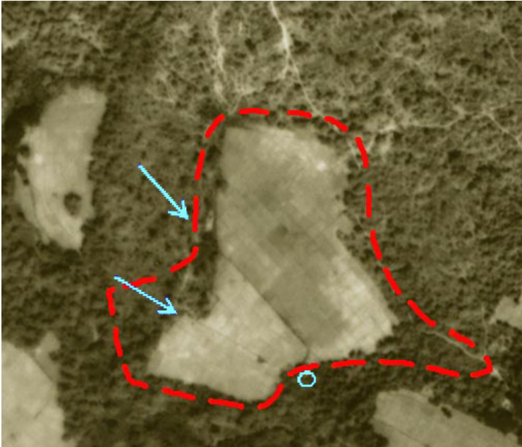
Fig. 3.1-14: Archive aerial photograph taken on February 1, 1945, showing a rice field near the city of Chiang Mai in northern Thailand. Irrigation ditches can be observed in the photograph within the rice field, which is now a waste disposal site. The ditches act as drainage system leading contaminants to the edge of the present-day landfill. Dashed red line: boundary of the waste disposal site. Arrow: direction of flow in the rice field's irrigation ditches. Blue circle: wet area at the edge of the waste site with assumed leachate. Archives research and acquisition by Luftbilddatenbank, Ing.-Büro Dr. Carls, Estenfeld, for BGR
