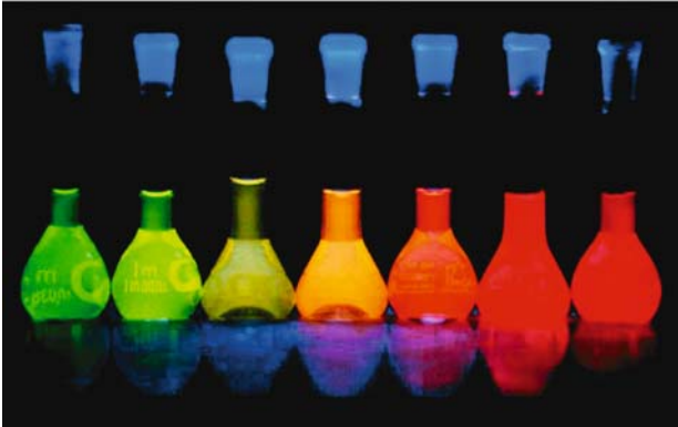
Fig. 13.31. Luminescence (under UV excitation) from flasks of colloidal CdTe quantum dots with increasing size (from left to right). From [458]
