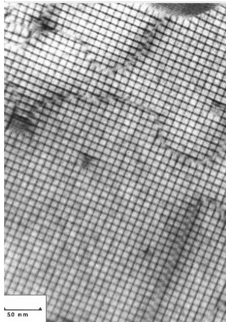
Fig. 4.13. Bright-field TEM image of pure twist boundary with network of pure twist dislocations fabricated by wafer bonding of two Si (001) surfaces with a relative twist. From [89]
