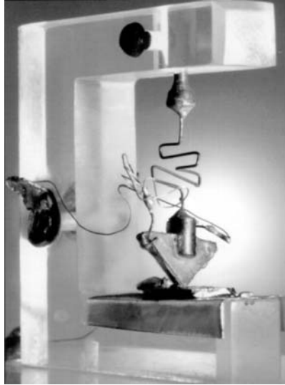
Fig. 1.4. The first transistor, 1947 (length of side of wedge: 32 mm)
