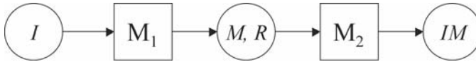
Fig. 10.1 The multi-component model representing EWS. M_1 is the earthquake prediction model and M_2 is the ground motion attenuation model
