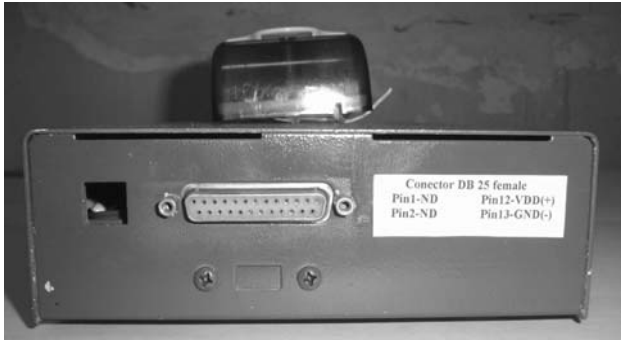
Fig. 17.5 Device configured to trigger at eight different levels following the user's requirements.
