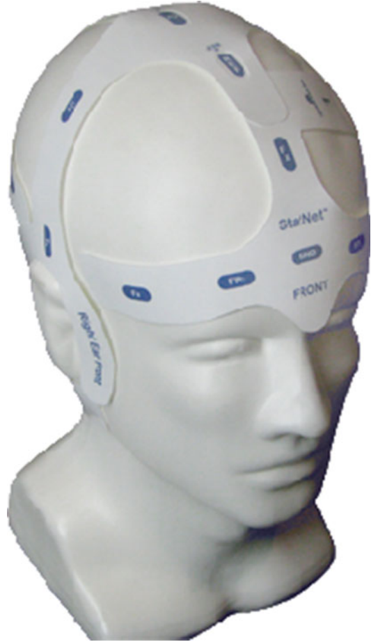
Fig. 2.8 Example of a disposable auto-adhesive EEG device (StatNet™, HydroDot Inc., reprinted with kind permission)
