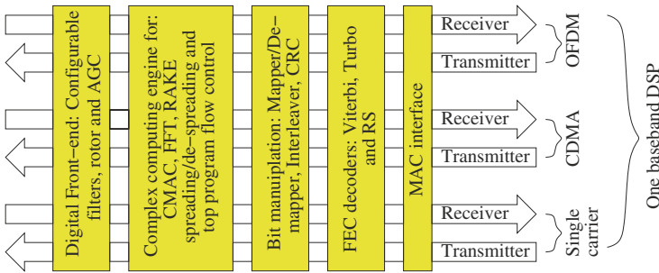
Figure 5.4. Hardware multiplexing on LeoCore DSPs.
