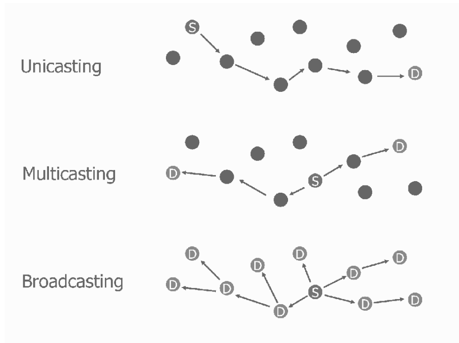
Figure 2.7. Illustration of unicast, multicast, and broadcast routing. S and D represent the source and destination nodes, respectively.
