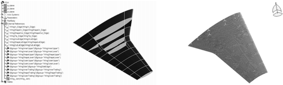
Fig. 3. Geometry of a structural wing model and FEM-model of the same wing
