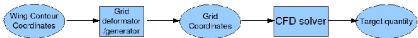
Fig. 1. Aerodynamic design chain. Oval boxes denote data and rectangular boxes numerical operations.
