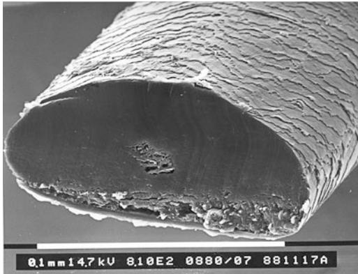
Fig. 17 Cross section of normal Caucasian hair with a discontinuous medulla ( center ). The cut through the fiber caused a disorder of the cortex material when the compression forces of the cutting edges were released ( bottom of fiber ). White bar 0.1 mm
