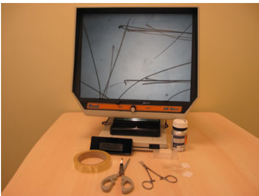
Fig. 1 Materials for the trichogram: microfilm reader, glass slides, cover slips, mounting medium, tape, scissors, forceps with rubber-protected jaws, and micrometric slide
