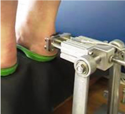
Fig. 3 Load application mechanism for applying intermittent normal and friction loads to the posterior aspect of the heel (Hashmi et al. 2013)
