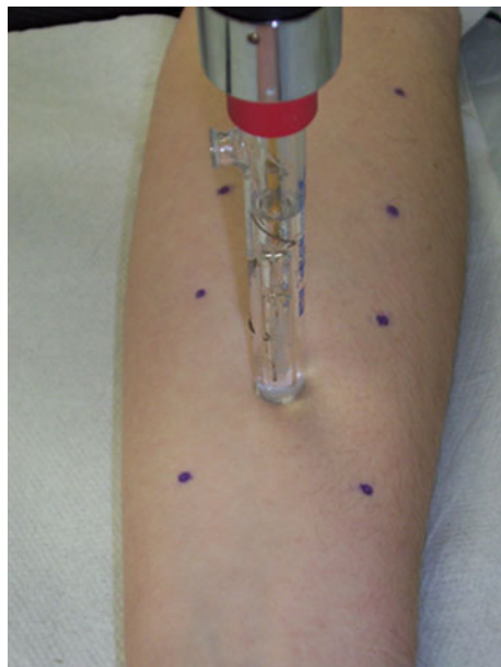
Fig. 1 Measurement of skin surface pH with flat glass electrode device Skin-pH-meter PH 905 (Courage and Khazaka electronic GmbH, Germany)
