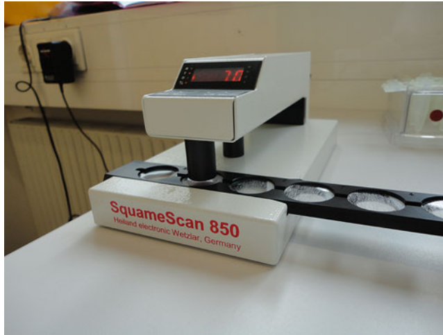
Fig. 2 The IR-densitometer SquameScan™ 850A (Heiland electronic GmbH, Germany) for analysis of SC proteins on adhesive tapes. The sample holders provide
