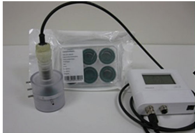
Fig. 8 The new ex vivo device. 1 Exposure chamber (donor compartment). 2 Thermostated jacketed. 3 Movable occlusion system. 4 Skin emplacement. 5 Diffusion cell (receiver compartment). 6 Magnetic stirrer
