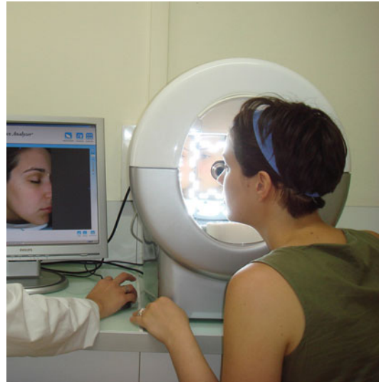
Fig. 4 Example of integrated system “light box” (Visioface ® , C&K). This independent comprehensive system consists of a box fitted with a camera, white light LEOs, chin and forehead rests to position the face, and image capture software. Homogeneous illumination is given by mirrors (visible inside the box) which distribute the light evenly on the face
