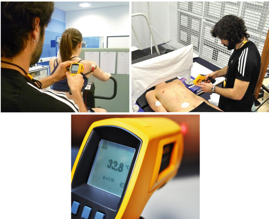
Fig. 16 The infrared thermometer used to measure local skin temperature before or after the contact with the stimuli
