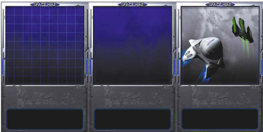
Figure 3-11. To clear the background, you simply draw a background sprite over the whole screen. Here are the three different background screens for Space Hike that are used: the main view, long-range scan view, and combat mode.
