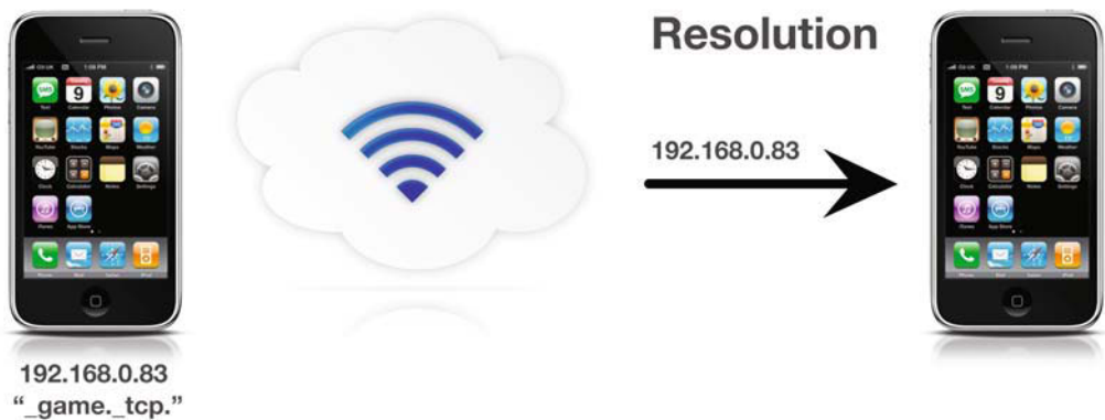
Figure 8-8. The service is resolved, so the devices can start communicating with each other.
