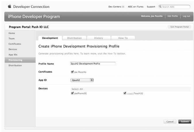
Figure 10-16. Set up the certificate, app ID, and devices for the development provisioning profile.
