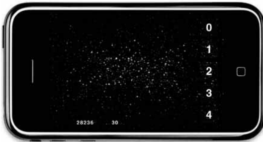
Figure 1-9. Boom! The SceneZero emitter after I hit it about 20 times in quick succession. Note the two numbers in the lower left. The big one is the number of particles, and the smaller one is the frame rate. I got this in the simulator. You would be hard-pressed to generate 28,000 particles and keep a 30 fps on the device.
