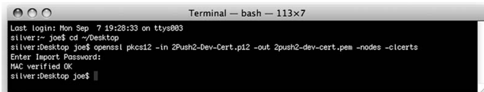
Figure 10-14. Convert the .p12 file to a .pem file for the server using openssl on the command line
