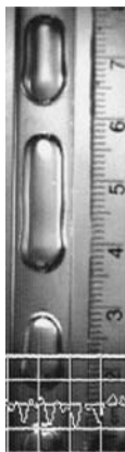
Figure 49. Flow image at \mu -g for flow 9. The \mu -g flow shows a series of rounded, smooth, uniform bubbles of approximately two to three tube diameters
