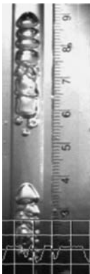
Figure 46. Flow image at 1-g for flow 8. The 1-g flow shows a trail of medium-sized bubbles. The leaders are compressed into ovals while the followers are stretched into irregular shapes. The tail has small spherical bubbles. A short liquid slug containing no bubbles separates the two groups
