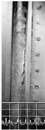
Figure 88. Flow image at 1-g for flow 15. The 1-g flow shows a similar frothy region at the bottom of the image and a notably irregular annular region at the top
