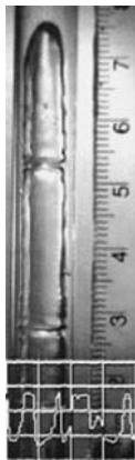
Figure 55. Flow image at \mu -g for flow 10. The \mu -g flow shows a long Taylor bubble with a rounded nose and a relatively smooth surface
