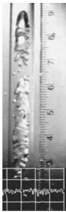
Figure 22. Flow image at 1-g for flow 4. The 1-g flow shows two separate trails of medium-sized bubbles. The bubbles are more closely packed and have diameters less than the tube diameter
