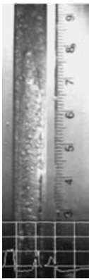
Figure 70. Flow image at 1-g for flow 12. The 1-g flow shows a distorted Taylor bubble. Many small bubbles are disbursed throughout the viewing section, particularly in the liquid slug in front of the Taylor bubble. The liquid slug is significantly longer than that for the \mu -g flow
