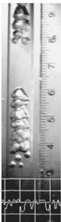
Figure 34. Flow image at 1-g for flow 6. The 1-g flow shows a trail of irregular shaped medium-sized bubbles. The small round bubbles at the end of the trail flow in a zigzag motion from the tube center to the wall and vice versa
