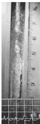
Figure 109. Flow image at \mu -g for flow 19. The \mu -g flow is annular with no complete breaks in the annular film. The smooth film is interrupted by the passage of a wave at the center of the image
