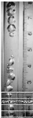
Figure 1. Flow image at \mu -g for flow 1. The \mu -g flow shows two separate trails of small rounded bubbles. The bubbles appear to flow near or at the tube center. The liquid slug separating them contains no bubbles
