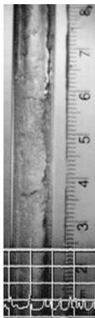
Figure 85. Flow image at \mu -g for flow 15. The \mu -g flow shows a frothy region in the center of the image, possibly the passing of a wave
