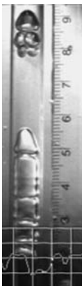
Figure 52. Flow image at 1-g for flow 9. The 1-g flow shows bubbles of one to two tube diameters forming clusters of varying lengths
