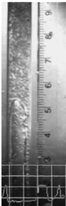
Figure 64. Flow image at 1-g for flow 11. The 1-g flow shows a similar situation where one long bubble follows the tail of another. However, this tail leaves a long trail of small dispersed bubbles in the long liquid slug
