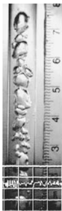
Figure 13. Flow image at \mu -g for flow 3. The \mu -g flow shows a packed trail of small bubbles with diameters less than one tube diameter. The bubbles flow at the center of the tube
