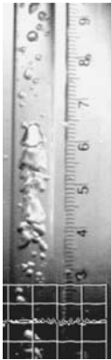
Figure 4. Flow image at 1-g for flow 1. The 1-g flow also shows a trail of medium-sized bubbles. In this case, the bubbles are packed more closely together causing the individual bubble shape to be flattened. The liquid slug is longer than in the \mu -g case and contains small dispersed bubbles. The void fraction is significantly greater than that at \mu -g
