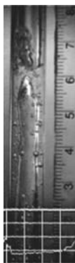
Figure 61. Flow image at \mu -g for flow 11. The \mu -g flow shows a liquid slug that separates two large bubbles. Small bubbles are disbursed in the thick liquid film. Few bubbles are present at the tail region of the slug
