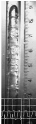
Figure 58. Flow image at 1-g for flow 10. The 1-g flow also shows a long Taylor bubble with many interfaces and rough edges. The nose is smaller in diameter
