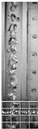
Figure 7. Flow image at \mu -g for flow 2. The \mu -g flow shows a loose trail of small bubbles. The bubbles are elongated in the direction of the stream flow. Very narrow liquid slugs separate small groups of bubbles
