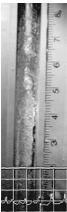
Figure 106. Flow image at 1-g for flow 18. The 1-g flow shows a more irregular film interrupted by decay of the annular flow and a frothy region with possible bridging
