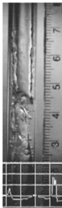
Figure 67. Flow image at \mu -g for flow 12. The \mu -g flow shows two Taylor bubbles touching nose to tail. The leading bubble has a slightly irregular film and the tail curves to mirror the rounded nose of the next bubble. A few small bubbles are disbursed in the narrow liquid slug that separates the two Taylor bubbles
