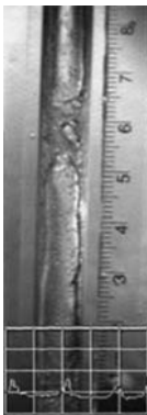
Figure 112. Flow image at 1-g for flow 19. The 1-g flow is interrupted by a frothy slug. It is difficult to determine if bridging is complete due to the presence of bubbles in the slug
