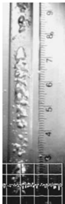
Figure 10. Flow image at 1-g for flow 2. The 1-g flow shows a more densely packed trail of irregular shaped bubbles. The liquid slugs preceding and following the trail contain small clusters of irregular shaped bubbles
