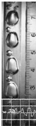
Figure 43. Flow image at \mu -g for flow 8. The \mu -g flow shows a repeating pattern of medium bubble – narrow slug – small bubble – narrow slug. The medium bubbles tend to be bell-shaped and flow at the center of the tube. The small bubbles are spherical and move toward the tube center
