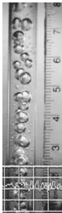
Figure 31. Flow image at \mu -g for flow 6. The \mu -g flow shows a group of spherical medium-sized bubbles together with some small dispersed bubbles. The bubbles tend to flow at or near the tube center
