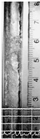
Figure 97. Flow image at \mu -g for flow 17. The \mu -g flow shows a frothy disturbance in the center of the image, this may be due to the passing of a wave
