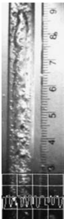
Figure 40. Flow image at 1-g for flow 7. The 1-g flow shows a distorted Taylor bubble. The bubble appears to break up near the bottom of the image into numerous small bubbles. Disbursed bubbles are seen throughout the viewing section
