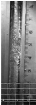
Figure 124. Flow image at 1-g for flow 21. Similarly, the 1-g flow also shows a disturbance at the center of the image, possibly the passing of a wave
