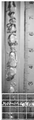
Figure 19. Flow image at \mu -g for flow 4. The \mu -g flow shows a trail of slightly distorted bubbles of approximately tube diameter length
