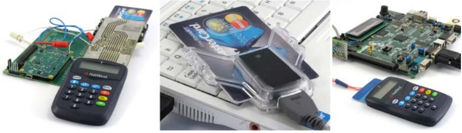
Fig. 2. We used FPGA boards to snoop on CAP transactions (left) and emulate a card (right). Using a USB card reader we emulated a CAP reader (centre).
