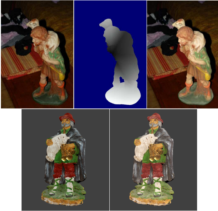
Fig. 6. Top: an example of color correction on a flash photograph: the original image (left); a normalized map of the offset correction on the image (center); the corrected image (right). Bottom: a colored 3D model, visualized with no illumination (only color values assigned to vertices). Color correction OFF in left image, ON in right one.
