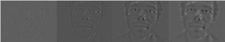
Fig. 7. Performing FRST by varying the subset of radii and fixed strictness parameter (radius increases). Dark and bright pixels are features with a high radial symmetric property.
