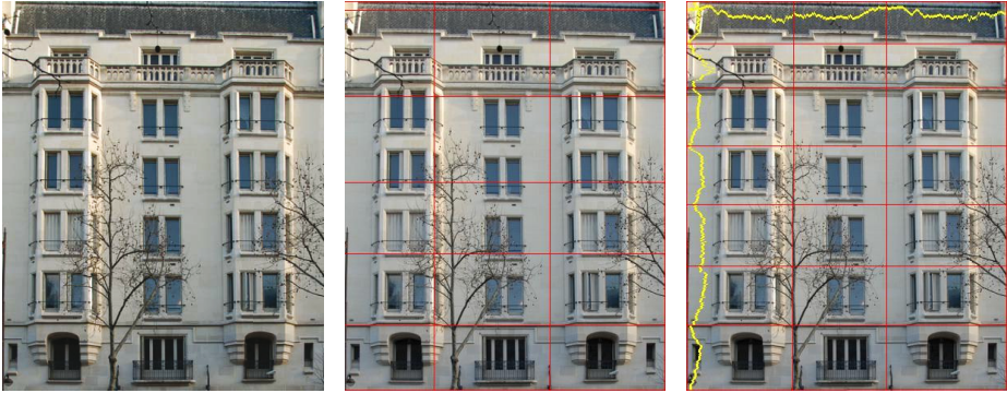
Fig. 5. Left: Original image with strong noise. Middle: Subdivision result using conventional MI-based method [17]. Right: Subdivision result using our method.
