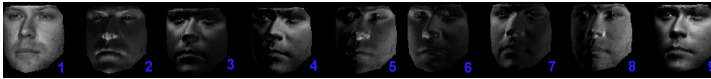
Fig. 3. Identity number 1 (from Yale database) illuminated by each one of the nine basis light sources
