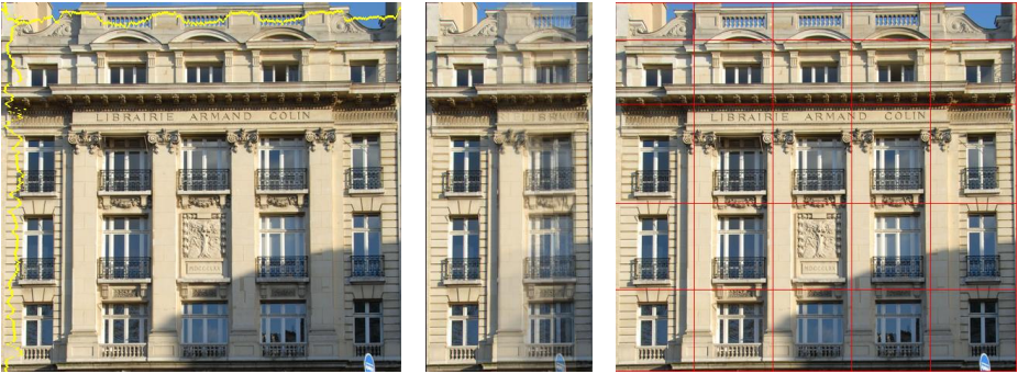
Fig. 2. Left: Original image with global edge profile in yellow. Middle: Tile templates. Right: Subdivision based on edge profile and GMI (splitting lines in red).
