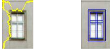
Fig. 3. Left: Tile edge profile in yellow. Right: Extracted window structure in blue.
