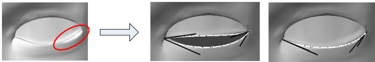
Fig. 6. Correction of the eyelid movement using deformable curves. Now the deformation of the eye boundaries is controlled by the curves and not by the FAP deformation function, so the eyelid matches exactly the under-eye boundary eliminating the problem illustrated in Fig. 2 c)
