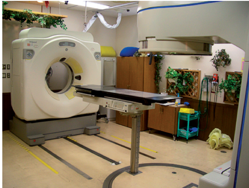
Figure 50 CT on rail-linac unit. A panoramic view of the integrated CT-linac irradiation system (a collaboration of Varian-Mitsubishi, Tokyo, Japan, and Yokogawa GE Medical, Tokyo, Japan). A linac gantry (on the right side of the figure) is placed on the opposite side of the CT gantry (on the left side of the figure). The common treatment couch is placed between these gantries. The treatment couch has two rotation axes for isocentric rotation to make noncoplanar arcs and for rotation between CT and linac. The CT gantry moved along a pair of rails on the floor and scanned the patient without sliding the table. The center of the CT image matched the isocenter of the linac accelerator when the couch was rotated 180°. The accuracy of matching the linac isocenter with the CT image center was within 0.5 mm.
