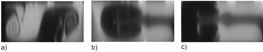
Fig. 11. Concentration distribution along the cross section, T-shaped micromixer 400x200x290, x=387\mu m , Re=160 , a) \dot{V}_1 = \dot{V}_2 , b) \dot{V}_1 = \frac{1}{2}\dot{V}_2 , c) \dot{V}_1 = \frac{1}{3}\dot{V}_2
