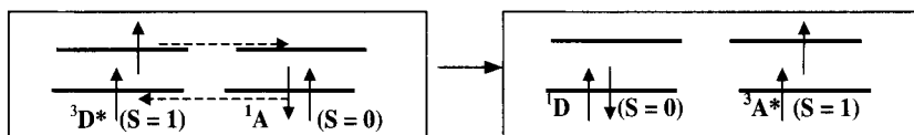
Figure VII-25. Dexter transfer with conservation of exciton state (example here is triplet): {}^3\text{D}^* + {}^1\text{A} \rightarrow {}^1\text{D} + {}^3\text{A}^* .
