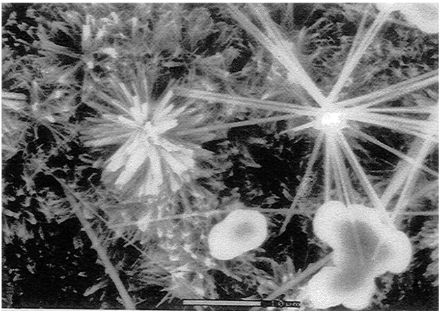
FIGURE 1-8 Secondary electron image taken in an environmental SEM showing long needle-like ettringite crystals and short “chrysanthemum-like” arrays of calcium-silicate-hydrate gel (C-S-H). Source: Hansson, 1995.
