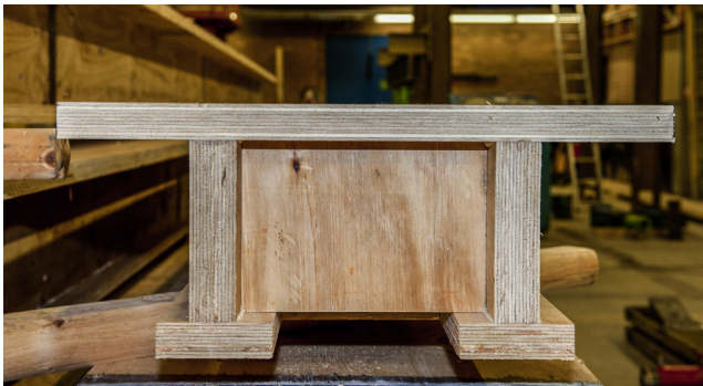
Figure 12.13 LVL composite beam with plywood gussets.
