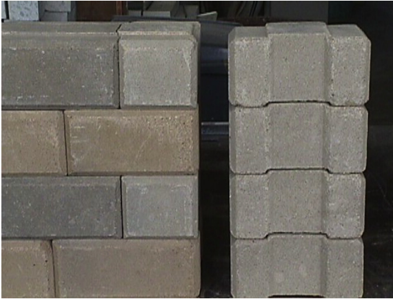
Figure 8.24 Front and side views of stacked blocks.
