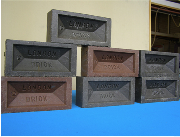
Figure 9.5 Unfired building bricks made with stabilized sulphate-bearing clay (Lower Oxford Clay, UK), using lime—GGBS blended binder (Industrial pilot-scale trials were carried out using a steel mould to make a well-known fired clay brick in the United Kingdom: ‘London’ brick, manufactured by Hanson Brick Company, Ltd.).
