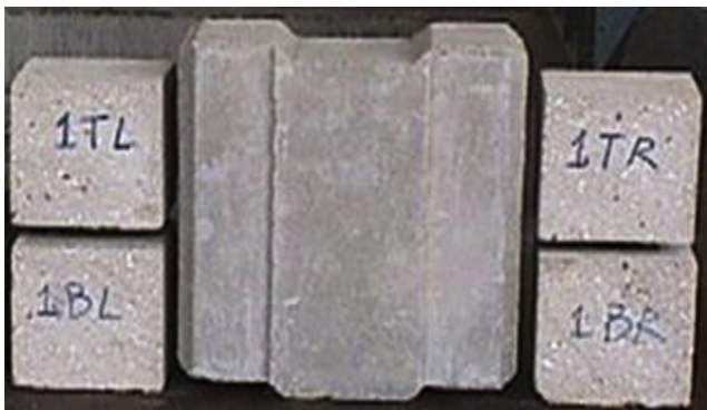
Figure 8.26 Hydraform block with cubes cut from a block.
