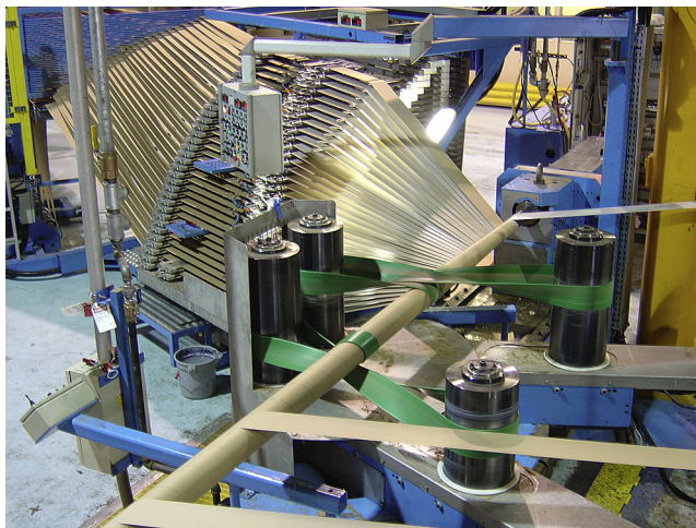
Figure 16.4 Paper tube manufacturing operation. With permission from Pakea.
