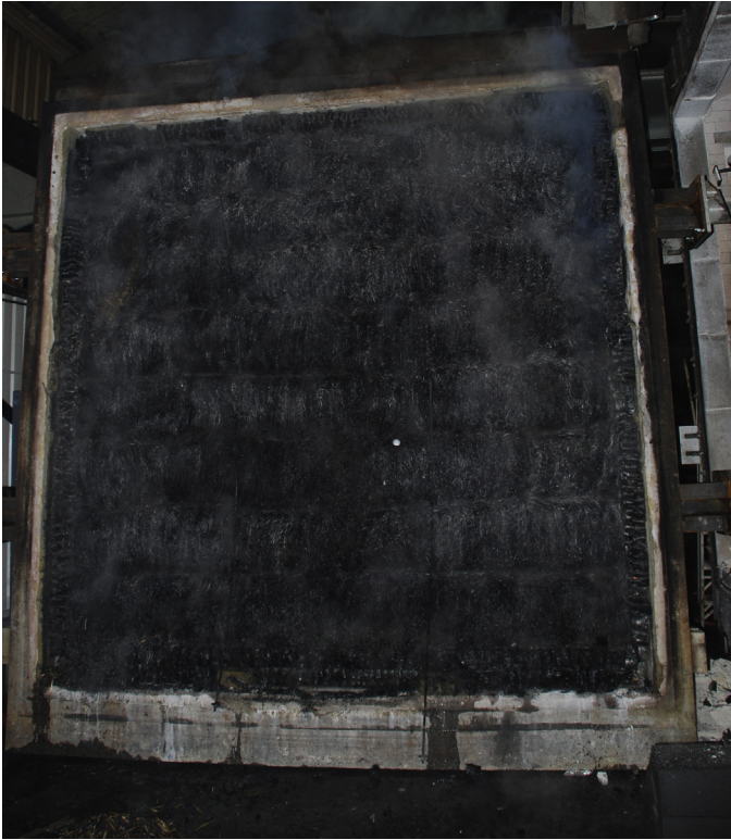
Figure 6.9 Straw bale panel after fire test.
