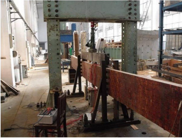
Figure 15.4 Static and fatigue loading test of full-scale glulam girder.
