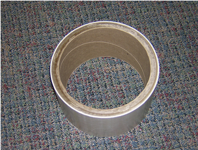
Figure 16.13 A 160-mm-ID, 16-mm-thick paper tube with an overmolded 3-mm pultruded outer layer.
