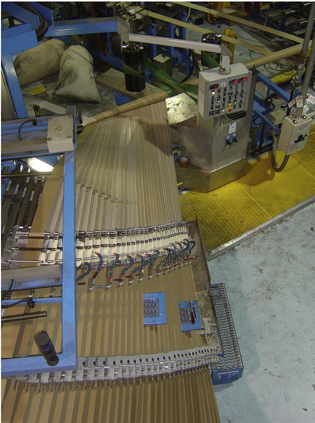
Figure 16.6 Ply positioning and adhesive application. With permission from Pakea.
