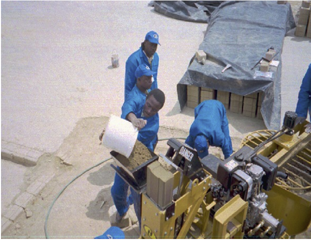
Figure 8.11 Soil-cement mix being loaded into the hopper. African Standards Organisation, 1996. Standards on CEB Construction: Compressed Earth Block Masonry ARS 670: Part 4: Code of Practice for Production and Construction.
