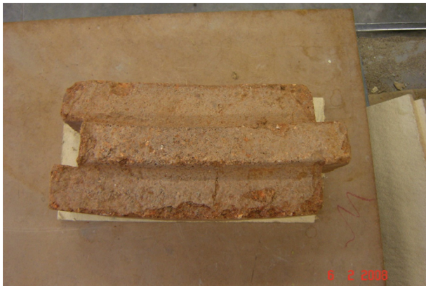
Figure 9.11 Innovative manufacture and applications of unfired clay materials. The curved blocks have been used for the construction of water tanks.
