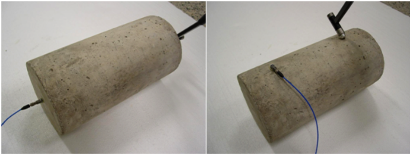
FIG. 4. Elastic wave test method (Left: ROD wave, Right: shear wave)
