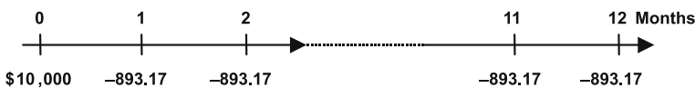
Figure 16.7 Cash-flow profile of an amortized loan with interest charged on outstanding balance
