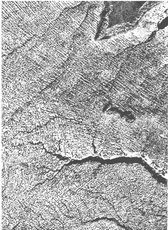
Fig. 1.4. Joint system in flat lying Entrada sandstone, Utah; aerial photograph, scale ca. 1:40000 (from D. Meier and P. Kronberg (1989) Klüftung in Sedimentgesteinen , Enke Verlag, Stuttgart)
