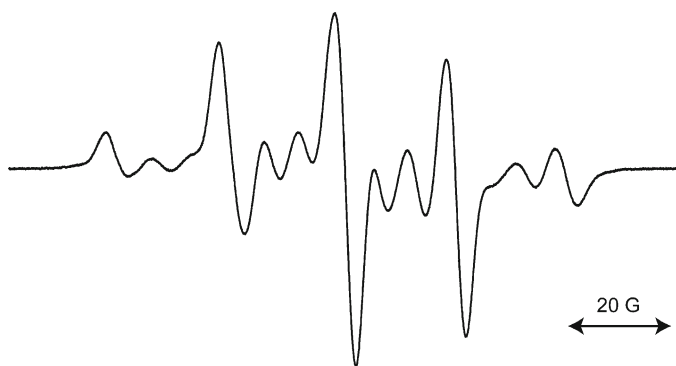
Fig. 9 ESR spectrum for propagating radical of Poly(methyl methacrylate) (PMMA) in the nanochannel of [\text{Zn}_2(\text{bdc})_2(\text{ted})]_n
