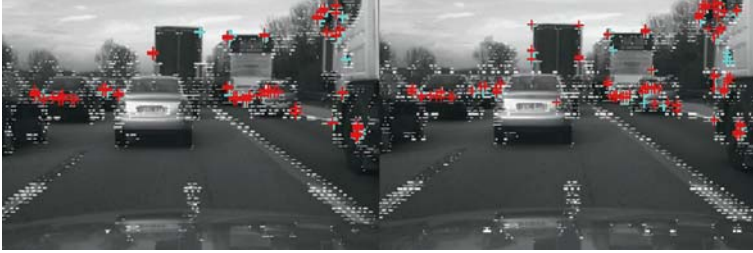
Figure 5.39. Corner candidates derived from regions with planar interpolation residues > 3\% (white bars) with parameters ( m , n , m_c , n_c = 3321 ). The circularity threshold q_{\min} = 0.6 eliminates most of the candidates stemming from digitized edges (like lane markings). The number of corner candidates can be reduced by lifting the threshold on the sum of the eigenvalues \text{trace}N_{\min} from 0.09 (right: 103, 121) to 0.11 (left image: 63, 72 candidates); cyan = row search, red = column search.
