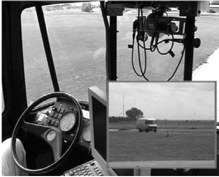
Figure 14.16. VaMoRs ready for mission demonstration 2001. The vehicle and road sections 1 and 8 (Figure 14.15) can be seen in the inserted picture. Above this picture, the gaze control platform is seen with five cameras mounted; there was a special pair of parallel stereo cameras in the top row for using hard- and software of Sarnoff Corporation in a joint project ‘Autonav’ between Germany and the USA.
