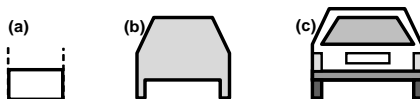
Figure 2.13. Coarse-to-fine shape model of a car in rear view: (a) encasing rectangle of width B (U-shape); (b) polygonal silhouette; (c) silhouette with internal structure
