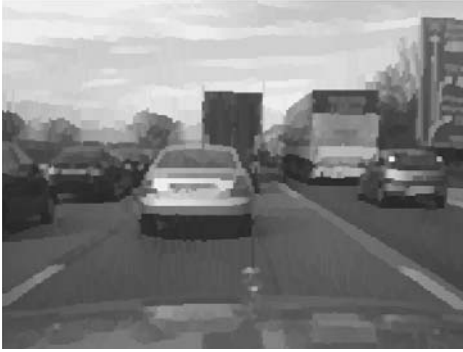
Figure 5.34. Image reconstruction for the parameter set (22.22) and vertical search direction, compressed horizontally 2:1 for display after processing. Scene recognition is no problem for the human observer
