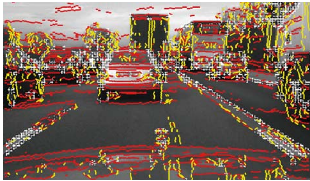
Figure 5.30. Edges from extreme values in gradient components in row (yellow) and column search (red, parameters m, n \cdot m_c, n_c = 33.21 ), \text{IntGradMin} = 0.016 ; white regions are bi-directionally nonplanar features.
