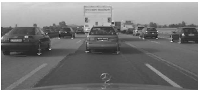
Figure 11.28. Confirming vehicle recognition under oblique viewing conditions based on characteristic wheel patterns. Area-based feature correlation in a 2-D search helps finding wheels by characteristic bright-dark patterns.
