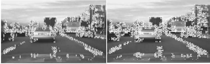
Figure 5.27. Nonplanar features for parameter set \text{ErrMax} = 2.5\% , mask elements m = n = 2 and cell size n_c = m_c = 2 (i.e., first pyramid level, left; after processing compressed 2:1 in rows for better comparison). Changing m_c to 4 (right) yields about the same number of features : \sim 2500 .
