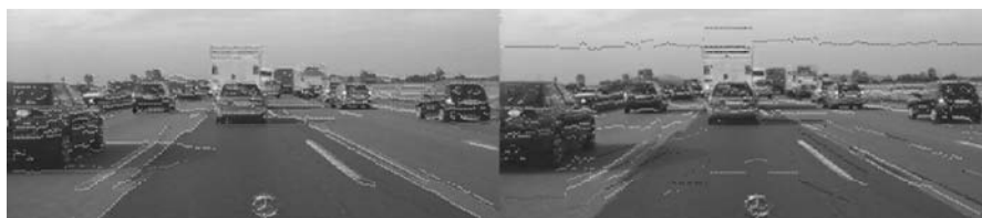
Figure 11.27. Example of joint detection of edges (left) and homogeneous regions (right) in vertical search with ‘Hofmann operator’. The vertical centers of homogeneous regions are marked with different colors [Hofmann 2004].
