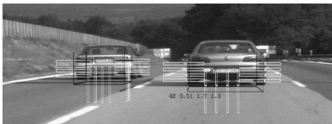
Figure 11.24. Object tracking with a COTS-PC system at the turn of the century. The software system applied for intelligently controlled edge extraction was CRONOS.
