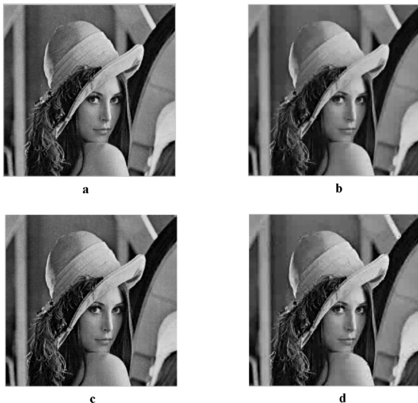
Fig. 13.8 Reconstructed Image, Lena. (a) Original Lena, 256 \times 256 pixels. (b) Reconstructed by (DCTQ-IQIDCT) Matlab (29.9 dB). (c) Verilog (DCT-IDCT) (38.9 dB). (d) Reconstructed by (DCTQ-IQIDCT) Verilog (29.4 dB)
