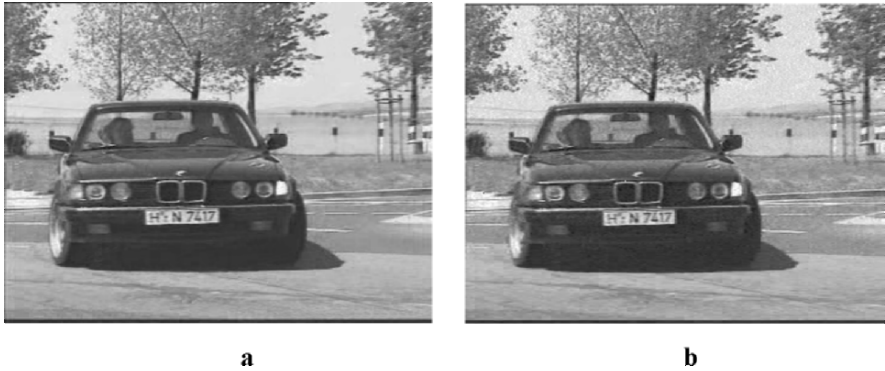
Fig. 11.14 Simulation image using FOSS motion estimation algorithm. (a) Original bmw image (frame number: 91, picture size: 352 \times 288 pixels) (b) Reconstructed bmw image by the FOSS method (PSNR: 35.6 dB)
