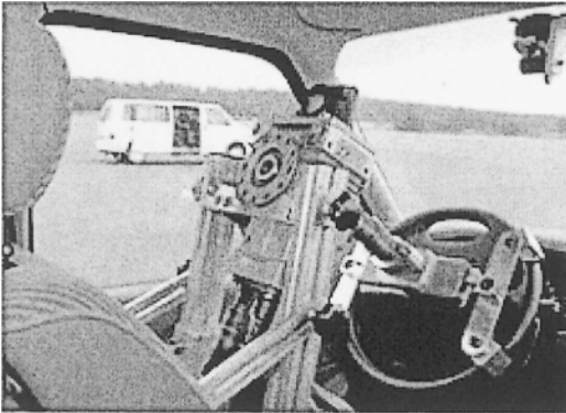
Fig.1.3 "Klaus," the driving robot developed by German carmaker Volkswagen, drives a VW Multi-van on a test track, from http://www.vw-personal.de/ .
