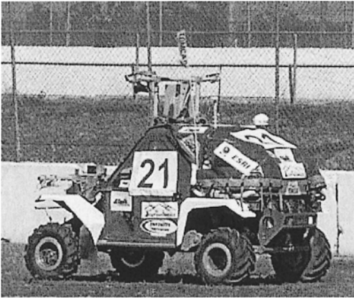
Fig.1.2 AVIDOR-2004 drives on the California Speedway QID track in Fontana, from [32]. The control system relies primarily on a differential GPS (Starfire) and a set of inertial sensors for navigating between the given set of waypoints. It uses infrared laser (LIDAR) and ultrasound sensing to provide the capability of obstacle avoidance and path following. (© [2004] IEEE)
