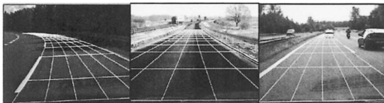
Fig.8.2 Three frequently encountered problems: (left) lane detection on roads with high horizontal curvature and shaded lane markers; (middle) lane detection on non-flat roads with vertical curvature; and (right) lane detection with the presence of obstacles on current lane; from [53]. (© [2004] IEEE)
