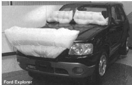
Fig. 3.13 Airbags used to prevent pedestrian injuries. Top row shows cowl airbags without (left) and with additional rear-rising bonnet (right). A vehicle equipped with over-the-bonnet and cowl airbags is shown on the right [Ford 2003, Autoliv 2003, Mazda 2003].
