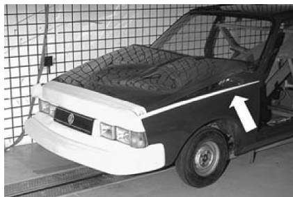
Fig. 3.12 Already in 1983 the Working Group on Accident Mechanics at ETH Zurich developed a rear-rising bonnet and showed its effectiveness (top row). The picture on the bottom row illustrates a model as it is introduced in current vehicles [Autoliv 2003].
