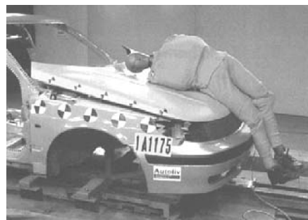
Fig. 3.12 Already in 1983 the Working Group on Accident Mechanics at ETH Zurich developed a rear-rising bonnet and showed its effectiveness (top row). The picture on the bottom row illustrates a model as it is introduced in current vehicles [Autoliv 2003].
