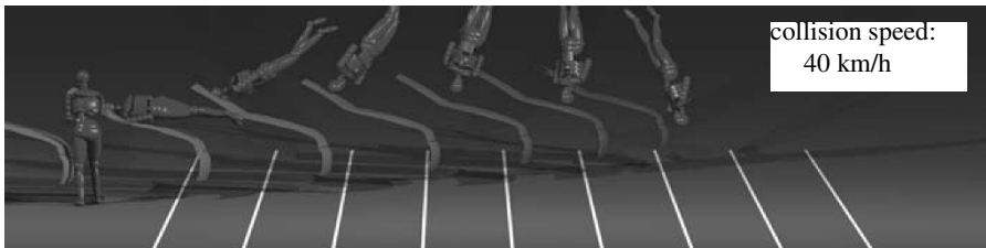
Fig. 3.14 Computer simulation of a pedestrian impact. The kinematics of the pedestrian change dramatically with increasing collision speed of the vehicle. This indicates that the secondary road impact has also to be considered [AGU 2003].
