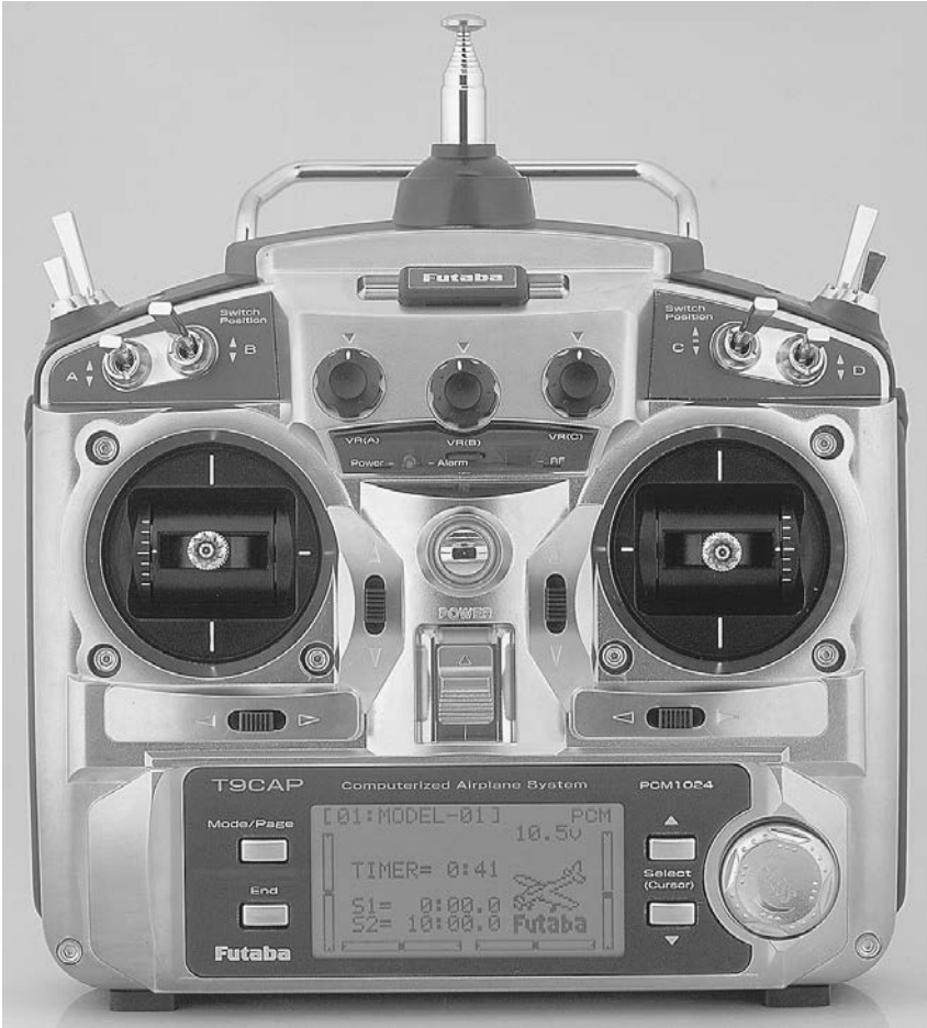
3.2 Radio control systems, operating on legal FM frequencies or in the 900 MHz radio band. COURTESY OF FUTABA CORP.
