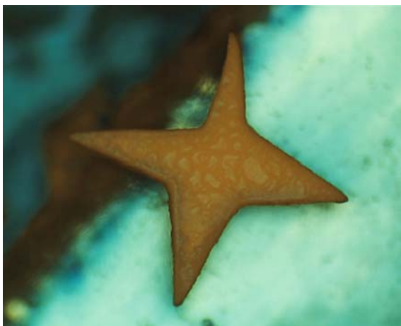
Fig. 4.7.5 Star-shaped polyNIPAM detached from the Si wafer after the FRRPP-based micropatterning operation using synchrotron X-rays
