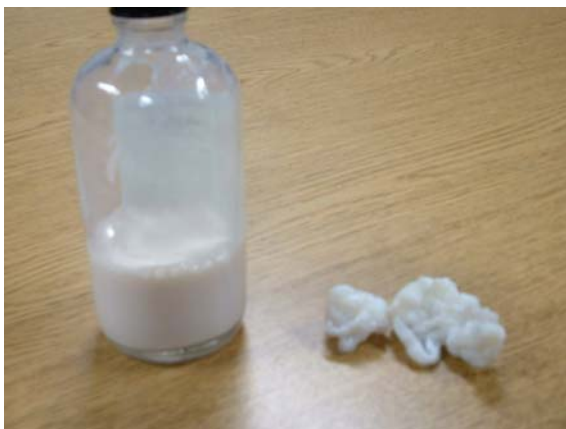
Fig. 3.2.5 Picture of a PS–PBA block copolymer emulsion and solid product made from a multistage FRRPP process with emulsification of the first-stage product
