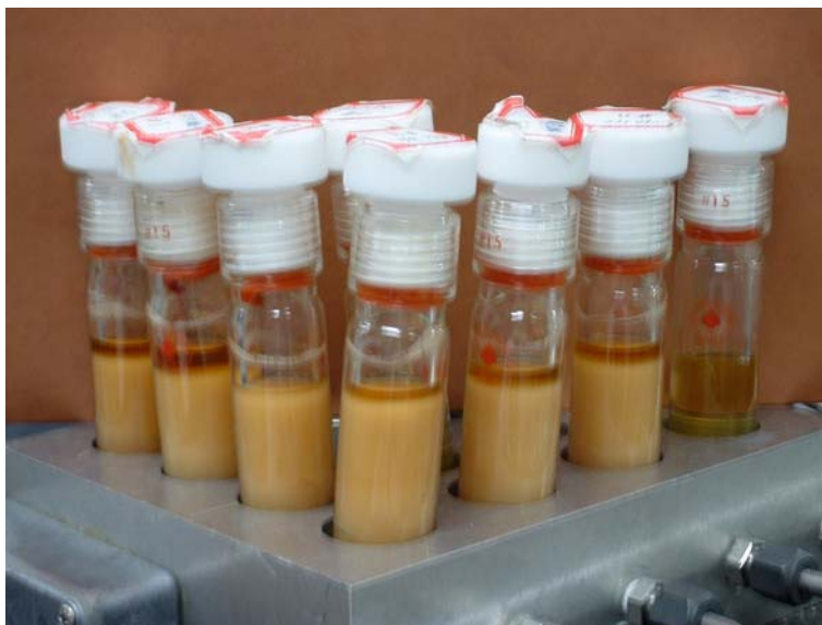
Fig. 4.2.2 High-throughput experimentation 10-atm glass tube reactors used in the early stage block multipolymer formation
