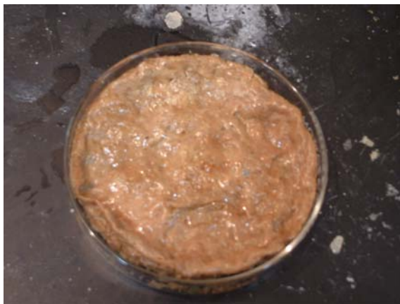
Fig. 4.3.3 Coagulated RB1-215 product on a Petri dish (With permission from Caneba et al., 2008)
