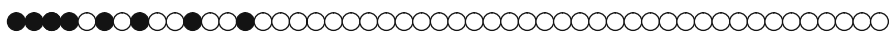
Fig. 4.6.5 Linear bead model of the vinyl acetate ( open beads ) and acrylic acid ( filled beads ) segments that make up the tapered B6-1 VA/AA block copolymer (see Sections 3.1 and 4.4). Bead numbers are drawn to scale to approximate molecular make-up of the blocky VA/AA material with 6 wt% AA segments
