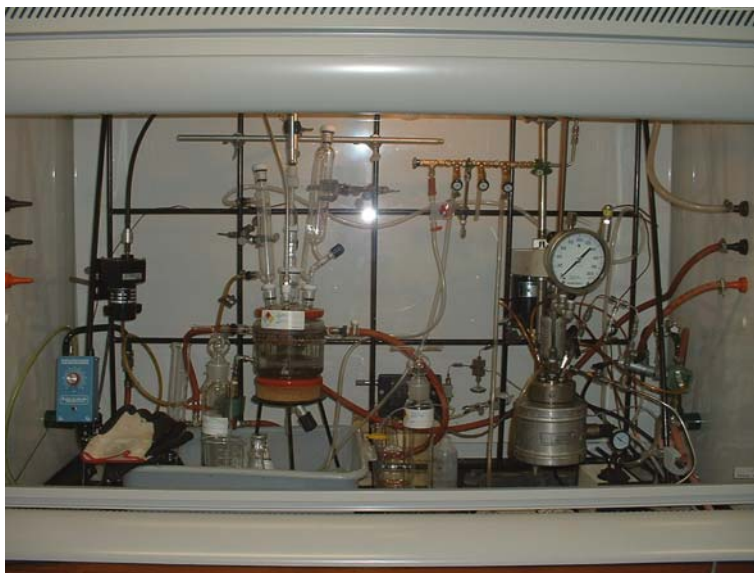
Fig. 4.2.1 First-stage stirred-tank reactor system (4,500 psig Parr reactor systems on the right) and second-stage 45-psig pressurized 1-l glass reactor on the left used to generate block multipolymers from radicalized VDC copolymer particulates (With permission from Caneba et al., 2008)
