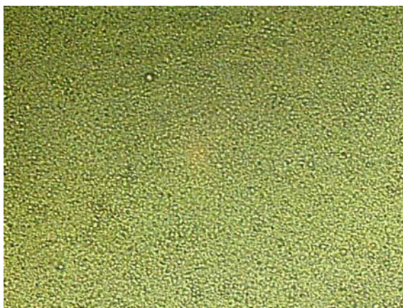
Fig. 5.2.4 Optical micrograph of a surface of a VA/AA-based emulsion (6.6 wt% solids) at 400X magnification, showing a bicontinuous network structure with 5–10 \mu\text{m} open cells (With permission from Caneba and Axland, 2002)
