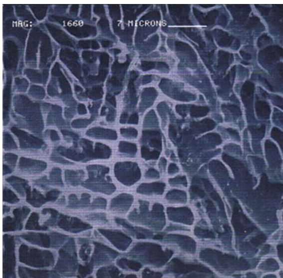
Fig. 1.4.37 Scanning electron micrograph of the pore structure of the PMAA membrane from a starting composition of 7%/3%/90% PMAA/MAA/water and quenched at 80°C for 2 min and 30 s (Reproduced with permission from Saxena, 2001)
