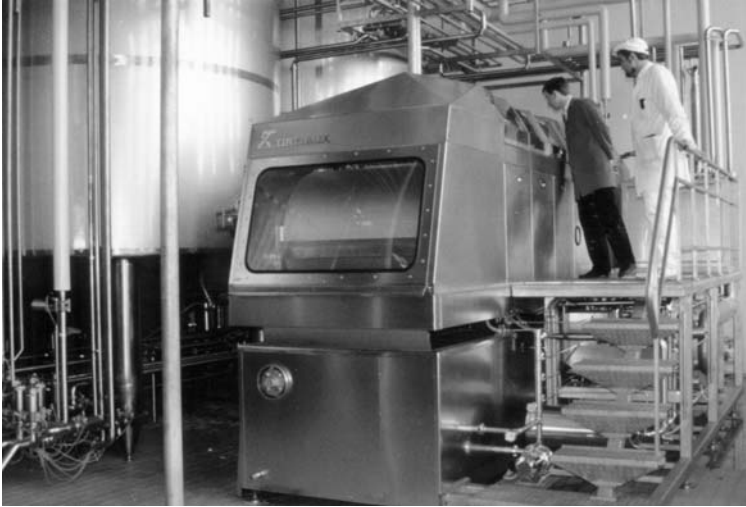
Figure 31 Florentine filter, shrouded and air-conditioned for cryofractionation.
