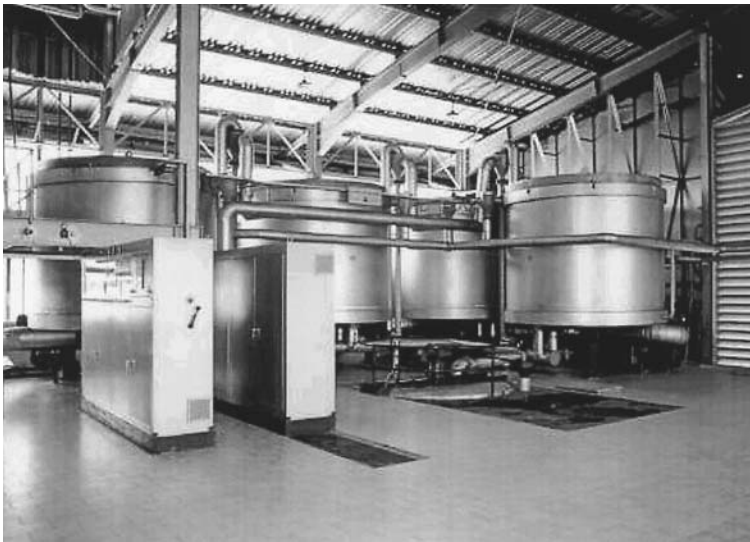
Figure 8 View of crystallizers in a de Smet fractionation plant. [Courtesy of Extraction de Smet N.V./S.A., Edegem (Antwerp), Belgium.]
