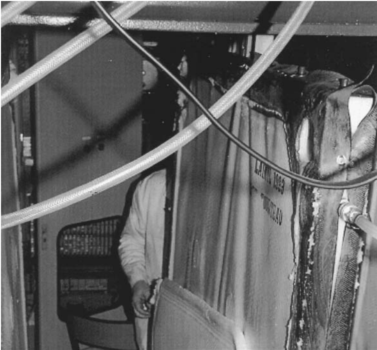
Figure 16 Membrane filter in a de Smet plant being opened for removal of the filter cakes. [Courtesy of Extraction de Smet N.V./S.A., Edegem (Antwerp), Belgium.]
