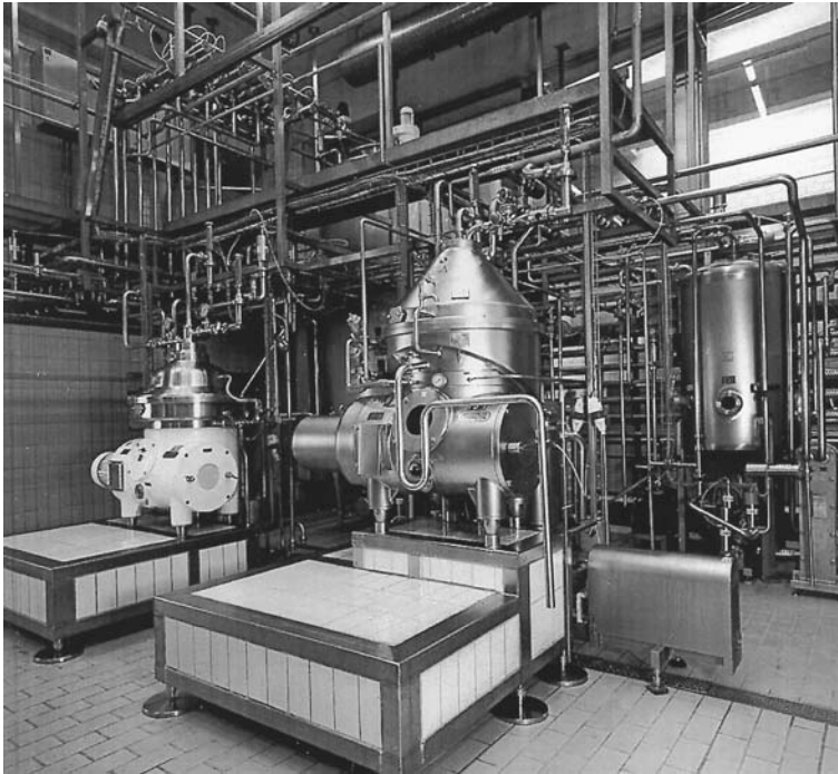
Figure 19 A nozzle centrifuge used for separating fat crystals from liquid oil. (Courtesy of GEA-Westfalia Separators, Oelde, Germany.)
