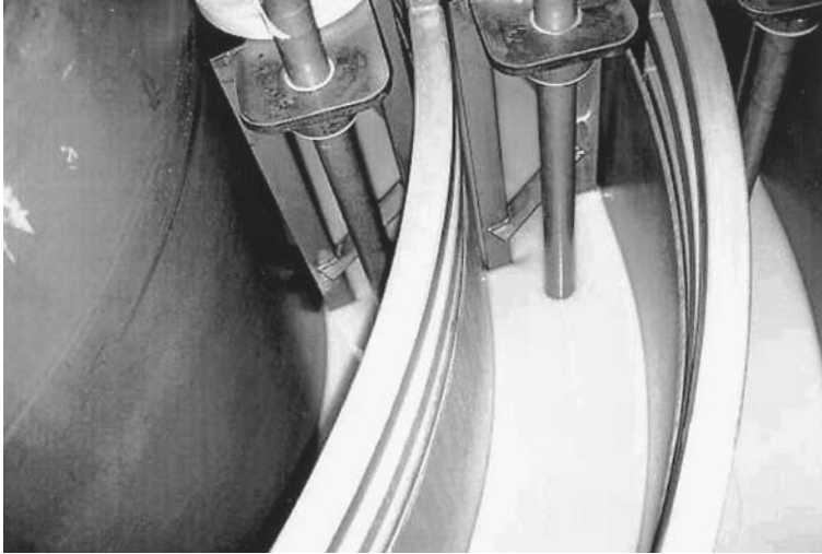
Figure 9 Detail of a de Smet concentric crystallizer. [Courtesy of Extraction de Smet N.V./S.A., Edegem (Antwerp), Belgium]
