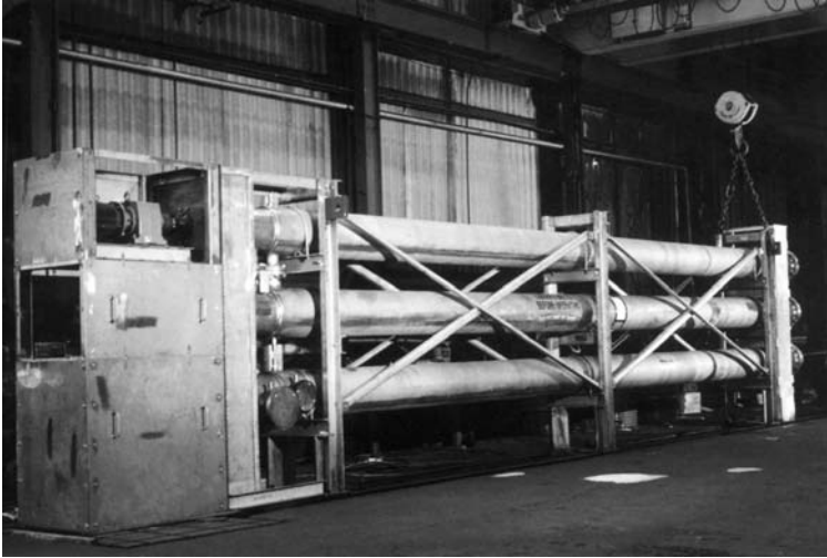
Figure 22 Armstrong-Chemtec scraped-surface crystallizer used in the solvent fractionation of fats. (Courtesy of Chemtec Pte. Ltd. Singapore.)
