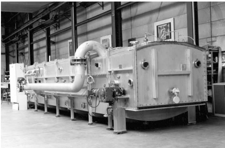
Figure 24 Pannevis continuous moving-belt filter for the solvent fractionation of oils and fats. (Reproduced courtesy of Pannevis BV, Utrecht, Netherlands.)
